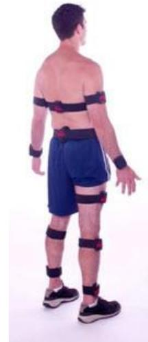
Fig. 22.3. Required sensor placements for the FAB system.
