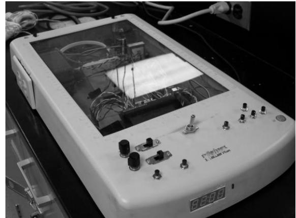
Fig. 21.1. The Sunrise Alarm Clock Prototype.
