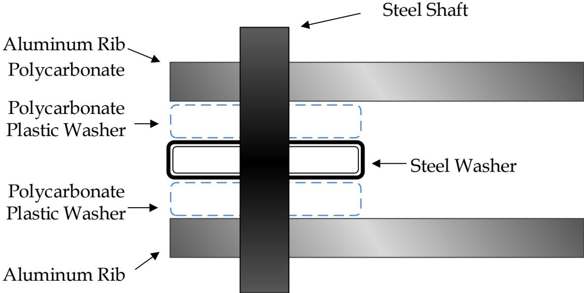
Fig.18.18. Cross section view of part of the pivot assembly.
