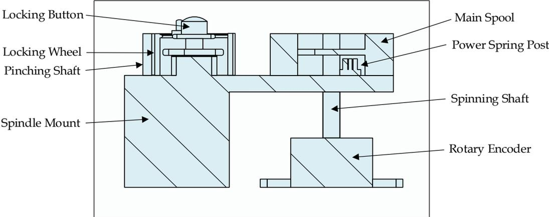
Fig.18.11. Section view showing interior components of Edema swelling measurement device.
