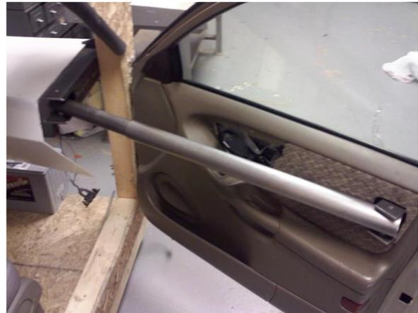
Fig.18.15. Vehicle Ingress/Egress Assistance Device.
