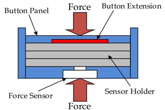
Fig.18.2. Cross section view of pinch sensing device.
