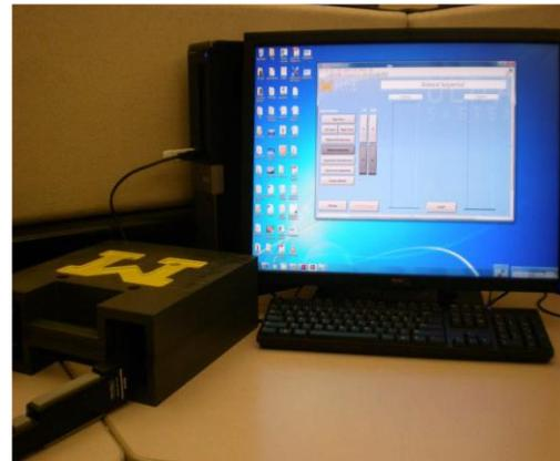
Fig.18.5. Hand Telerehab Device and Accompanying LabView program.
