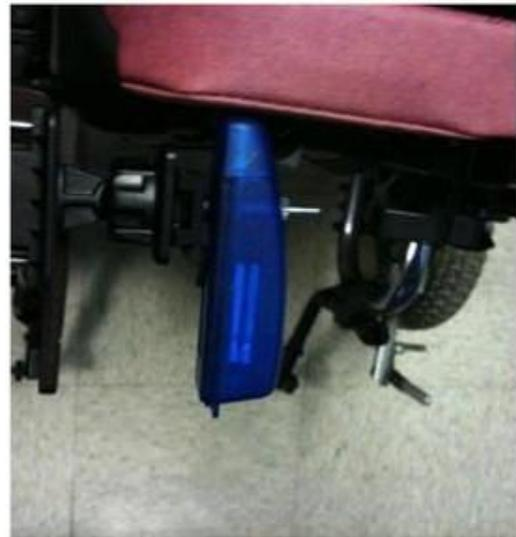
Fig. 16.5. Accelerometer mounted on wheelchair.
