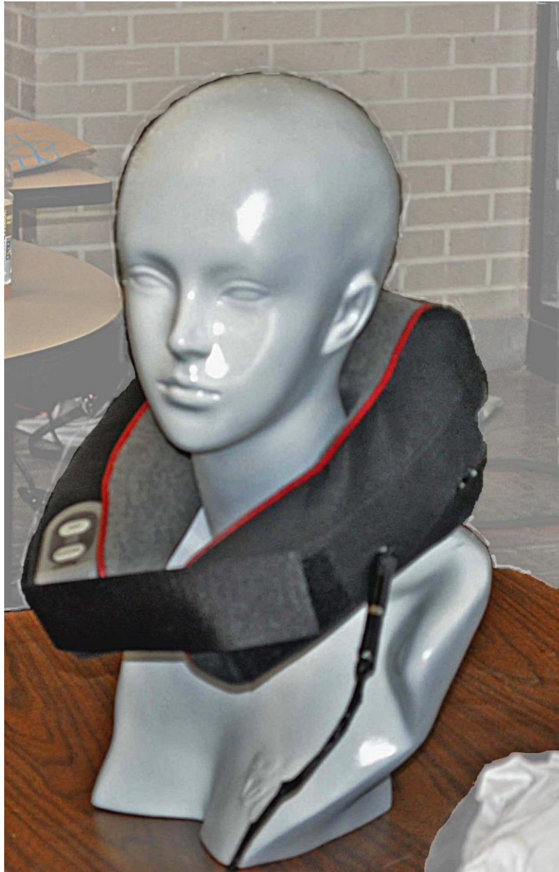
Fig.15.5. The stimulation device with button cable and connectors.
