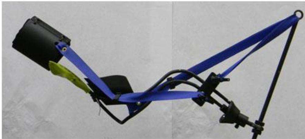
Fig. 10.12. Final Prototype of Mobile Arm Support.
