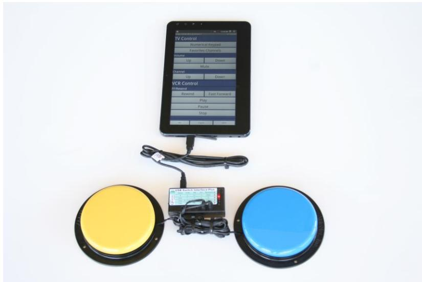
Fig. 9.7. Android Device with two button inputs.
