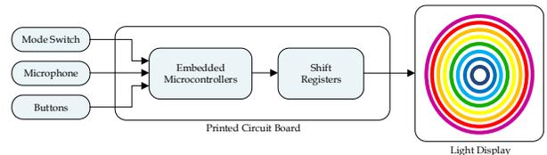
Fig. 9.3. Block Diagram.
