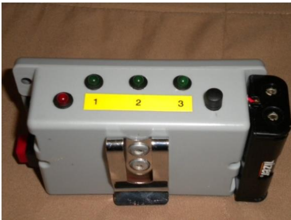
Fig. 8.17. Back – side view of the PAS showing indicator LEDs and battery pack.
