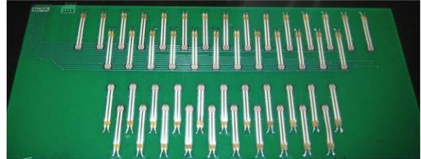
Fig. 9.7. Modified spring configuration for keyboard keys.
