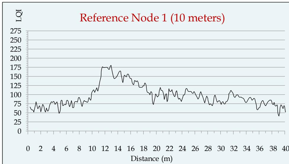
Fig. 21.8. Signal Strength between second and blind nodes
