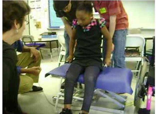
Fig. 17.7. The device lifts up the client as she de-weights herself.
