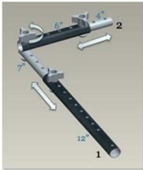
Fig. 14.4. CAD drawing of device.
