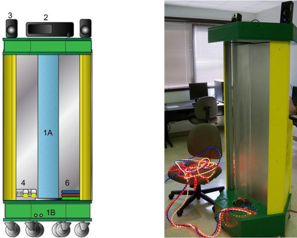
Fig. 14.2. (Left) Schematic and (Right) completed sensory stimulation device including: bubble tube (1A), interactive controls of the bubble tube (1B), projector (2), speakers (3), aroma therapy (4), tactile boards (5), and rope lights (6).
