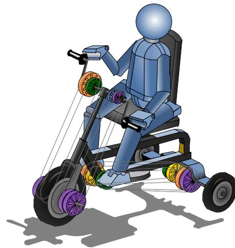
Fig. 9.8. Computer model of the adapted tricycle.
