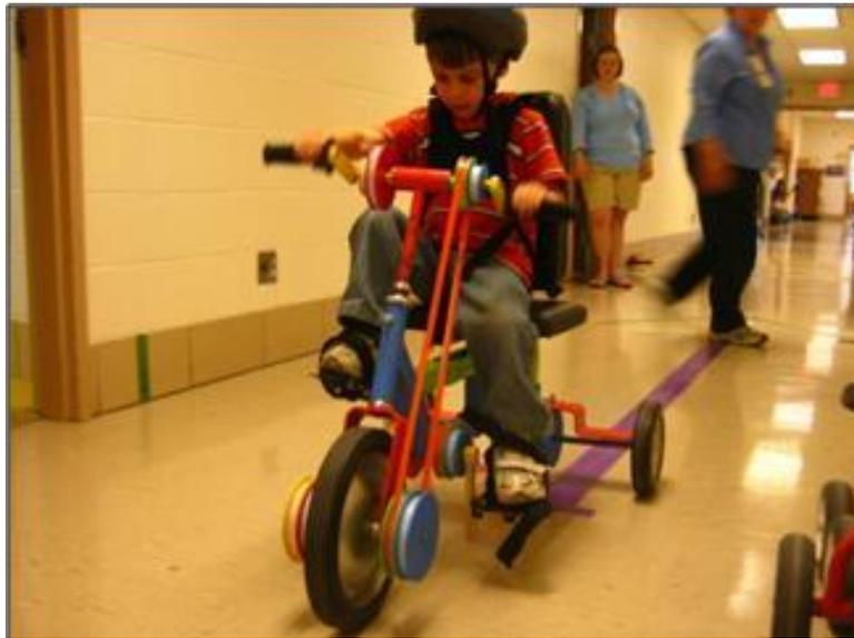
Fig. 9.10. Photo of completed adapted tricycle.
