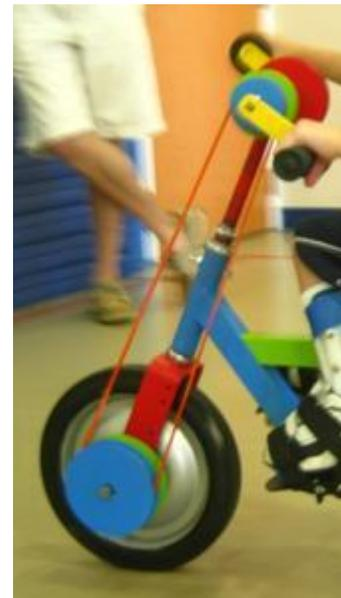
Fig. 9.9. Pulley and belt drive train.
