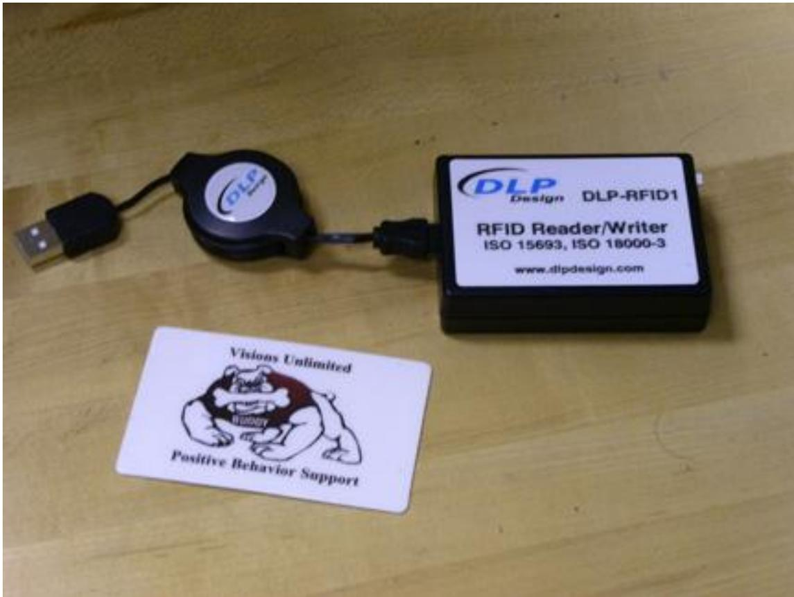
Fig. 23.6. The passive FID tag and the RF reader which connects to a PC via a USB cable.
