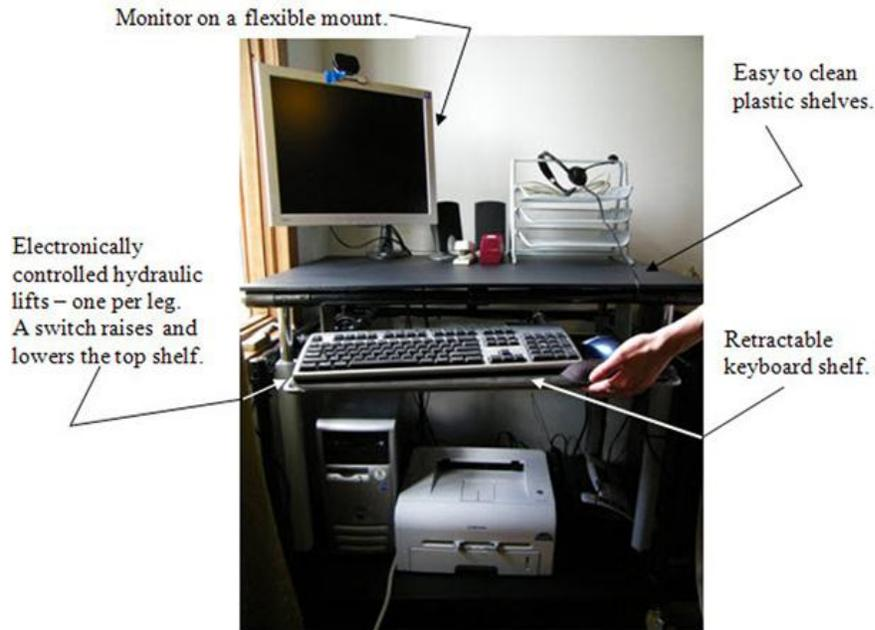
Fig. 23.3. The mobile adjustable computer station with casters.
