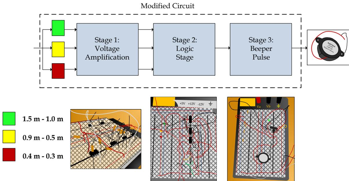
Fig. 22.9. Circuit schematic and breadboards for system.
