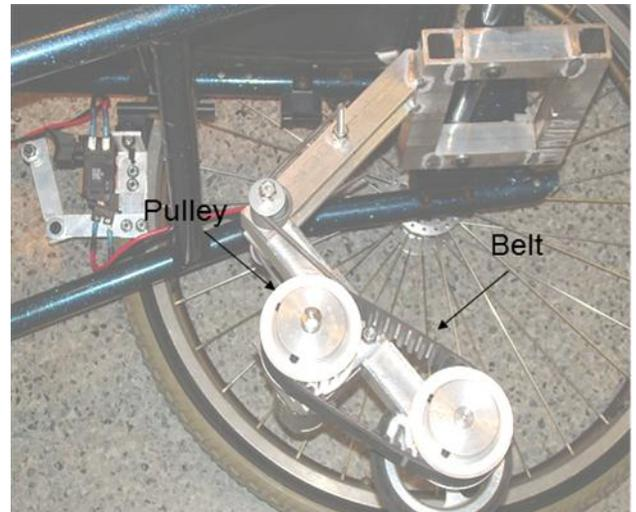
Fig. 22.4. Left Hand View of Augmentative Power Assembly.
