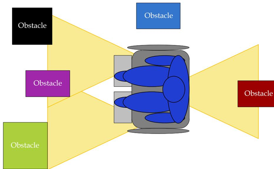
Fig. 22.8. Schematic of detection system - detection areas.
