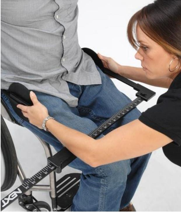
Fig. 22.2. Demonstration of calipers with pressure paddles used to measure hip width.
