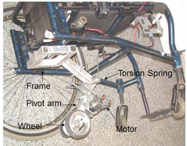
Fig. 22.5. Right Hand View of Augmentative Power Assembly.
