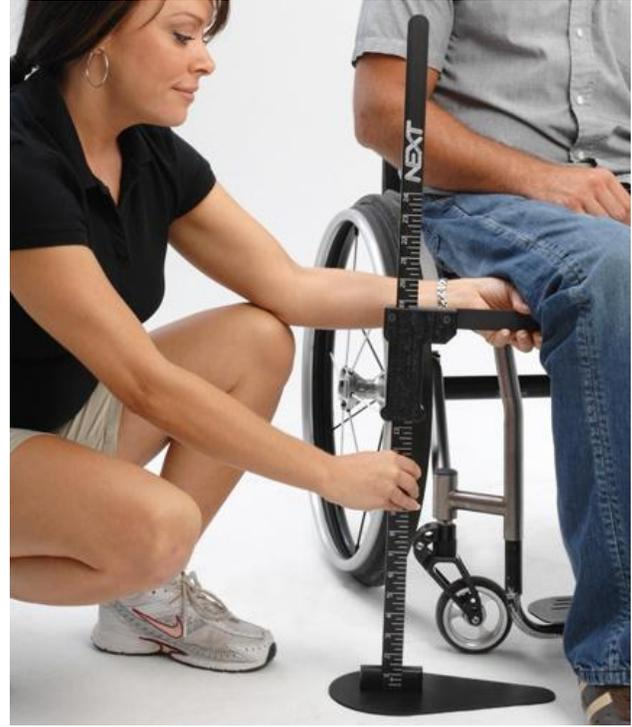
Fig. 22.3. Demonstration of height gauge with sliding caliper used to measure lower leg length.
