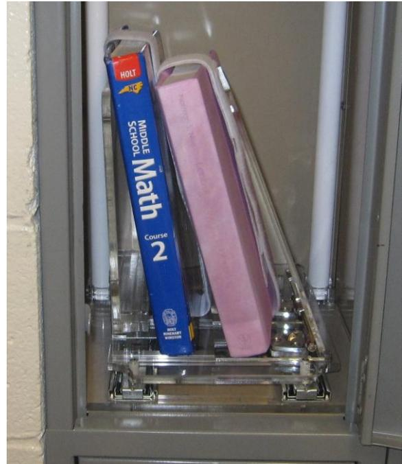
Fig. 20.3. The locker assist installed inside the client's locker.
