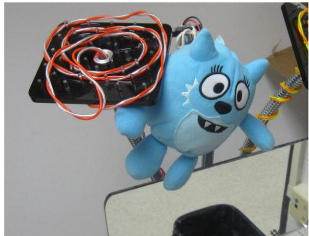
Fig. 20.6. Close up of the mirror [bottom right], electroluminescent wires [top left], and shaking toy [center].
