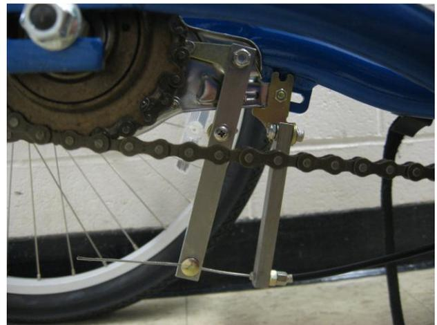
Fig. 20.8. The custom tricycle braking system (top) and close up of the extended lever arm for rear band brakes (bottom).
