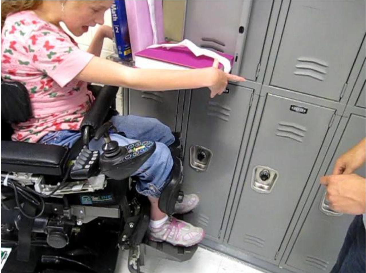
Fig. 20.4. The client places a book on the locker assist flap, and then rotates it to a vertical position.
