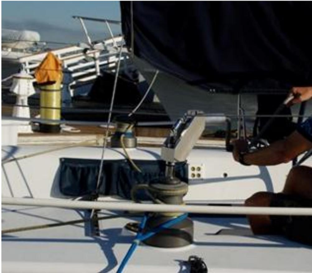
Fig.13.3. Winchtop grinder in use on racing sailboat.
