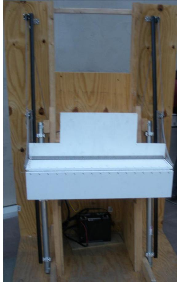
Fig. 13.1. Cabin lift system attached to mock-up of ladder.
