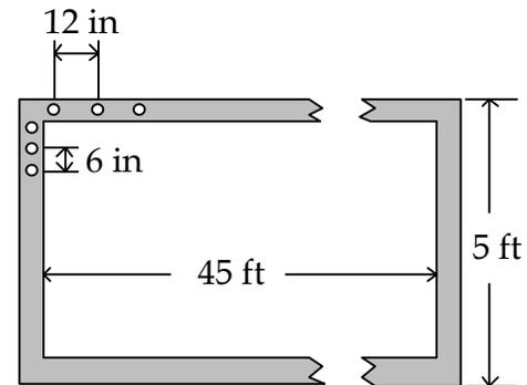
Fig. 12.10. Spacing of the holes along the Bubble Wall.
