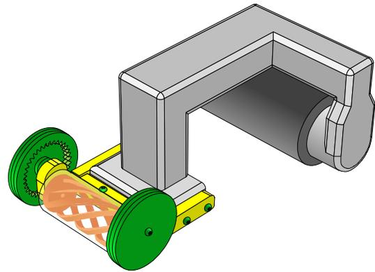
Fig.12.1. "Push Mower" design for thread trimming.
