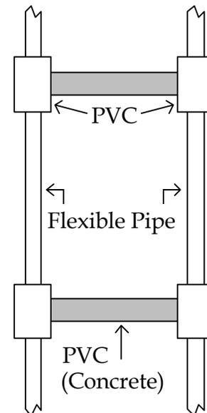
Fig.12.11. PVC Stabilizers for the Bubble Wall.
