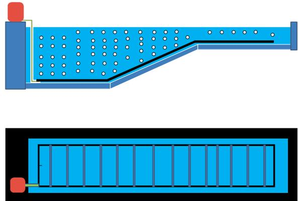
Fig. 12.12. Side (top picture) and bottom (bottom picture) schematic of the Bubble Wall.
