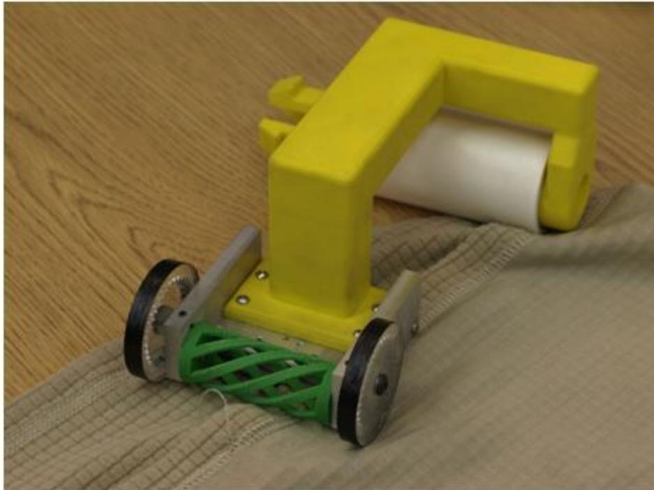
Fig.12.2. Final Prototype of the "Push Mower" design for thread trimming.
