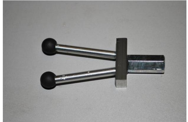
Fig.12.3. Modified headgear with two prongs for easy paper manipulation.
