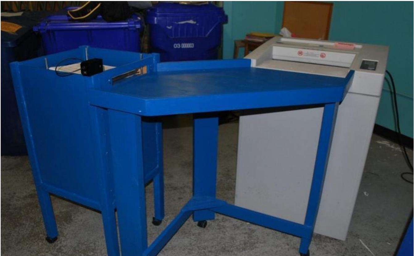
Fig.12.5. Spring box and guide way for improved access to the paper shredder.
