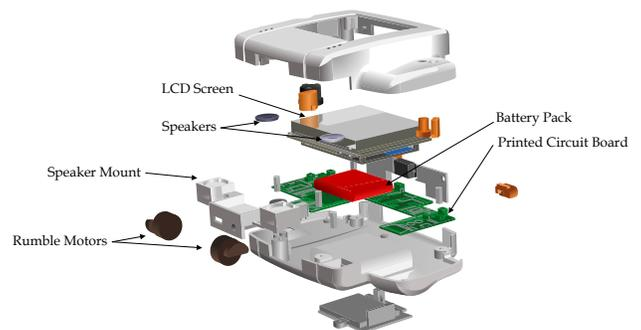
Fig.11.1. Custom designed handheld gaming device.
