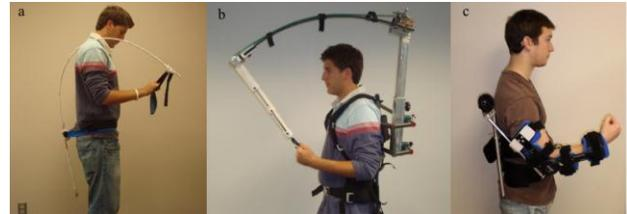
Fig. 11.6. Left to right: therapist prototype, first-generation exerciser, and present design.
