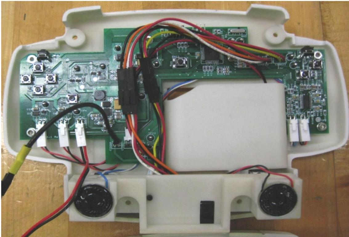
Fig.10.5. Interior of case with PCB mounted.
