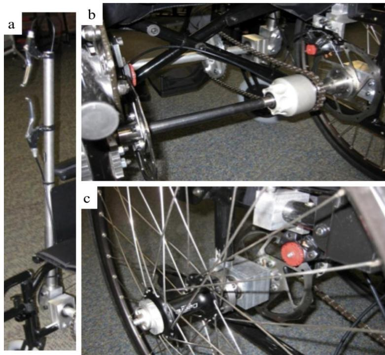
Fig.11.11. Key propulsion system components: (a) push lever and brake handles, (b) chain drive and differential, and (c) rear wheel hub and brakes.
