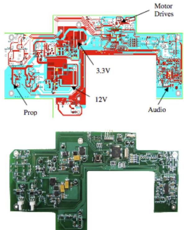
Fig.11.3. PCB layout (top) and final PCB (bottom).
