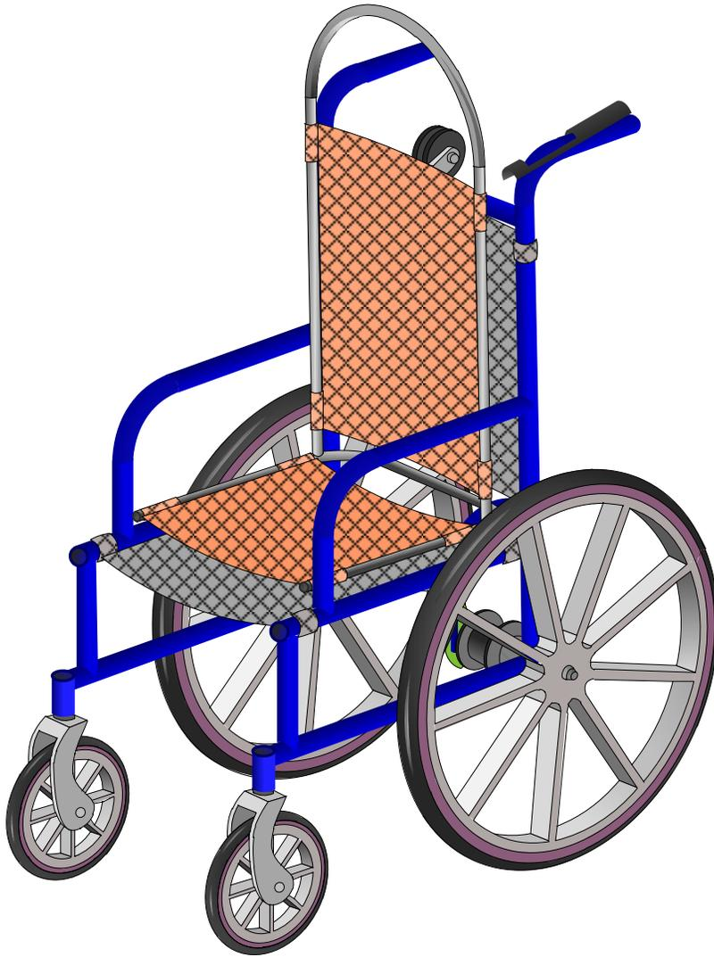
Fig.10.12. The computer model of the Lift Assist device.
