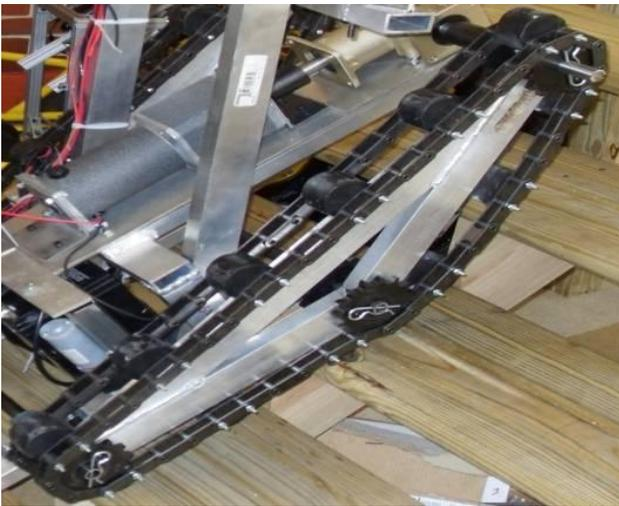
Fig.10.10. The treads of the device.
