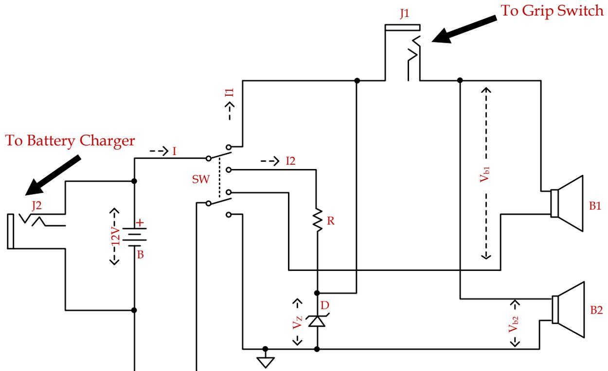
Fig. 17.11. Circuit schematic for sound box.
