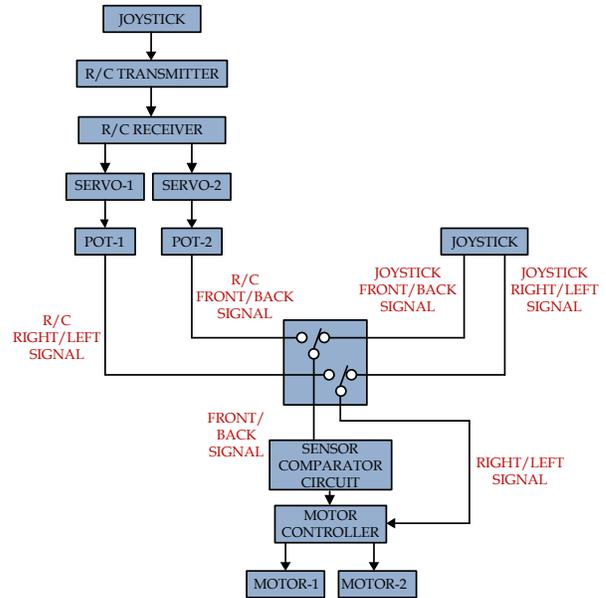
Fig. 17.2. Control diagram.
