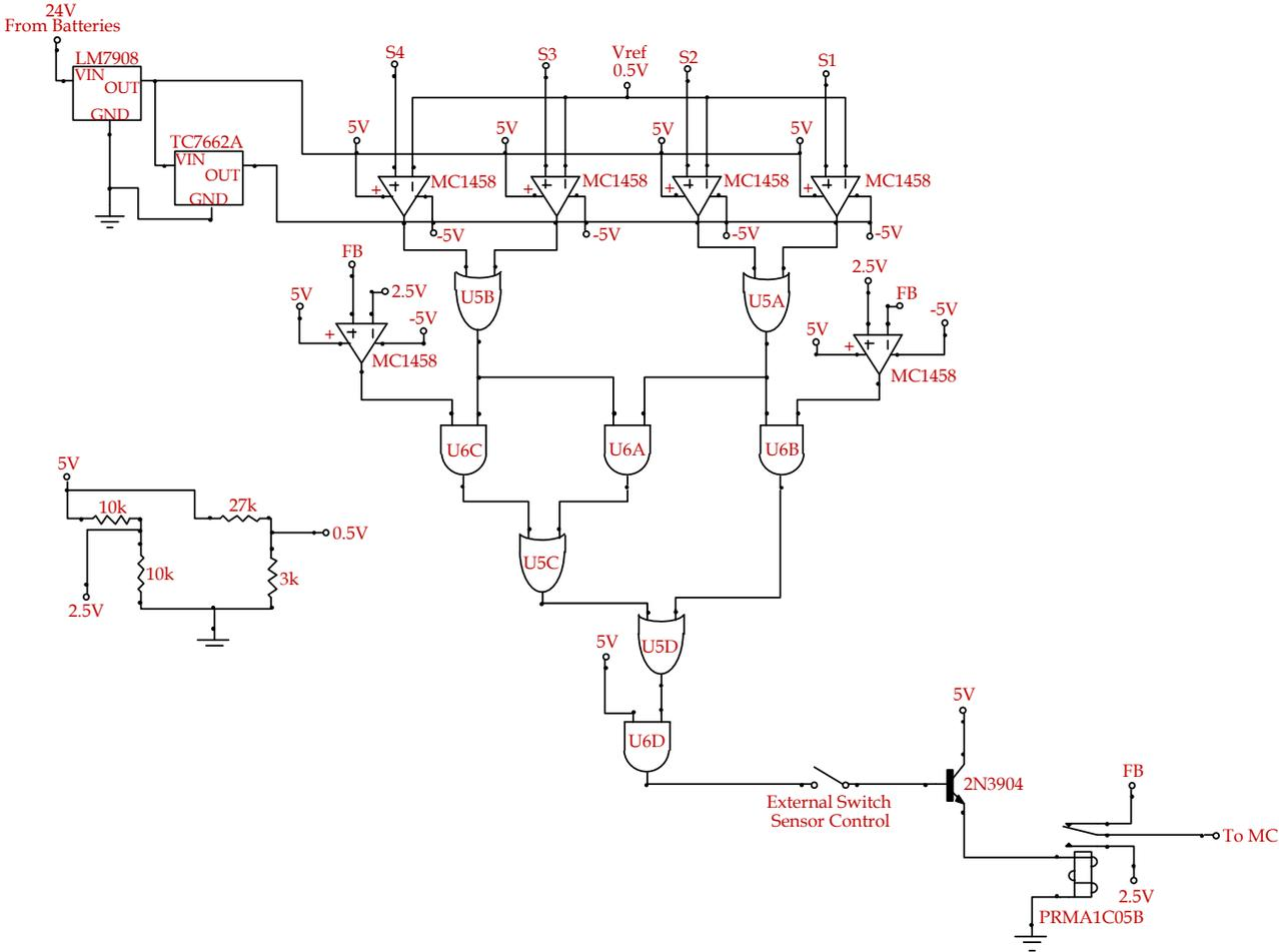
Fig. 17.3. Sensor control circuit.
