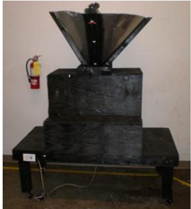
Fig. 17.4. The adaptive can crusher.
