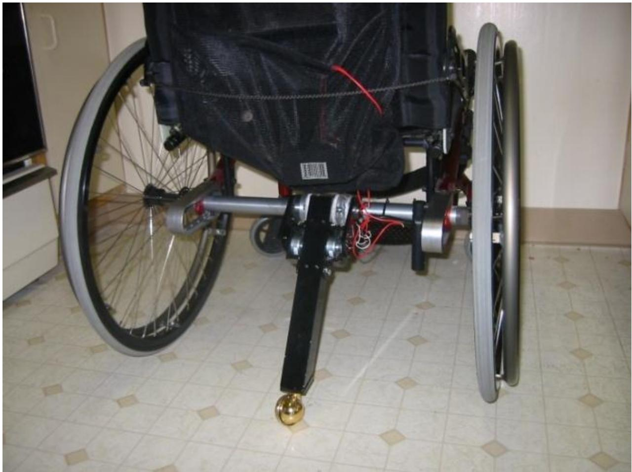
Fig. 15.9. New anti-tip system.
