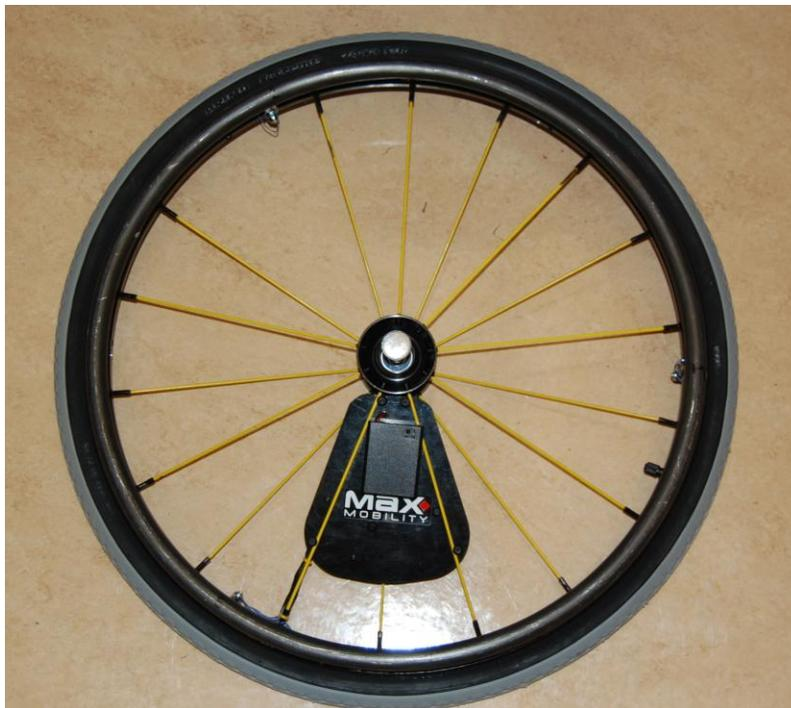
Fig. 15.7. The instrumented wheel prototype.
