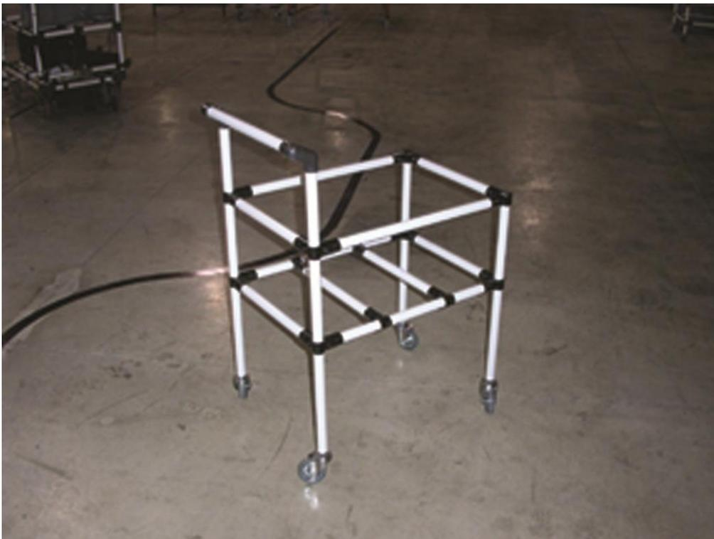
Fig. 20.5. Custom-Designed Delivery Cart for Raw, Unpainted Tools.
