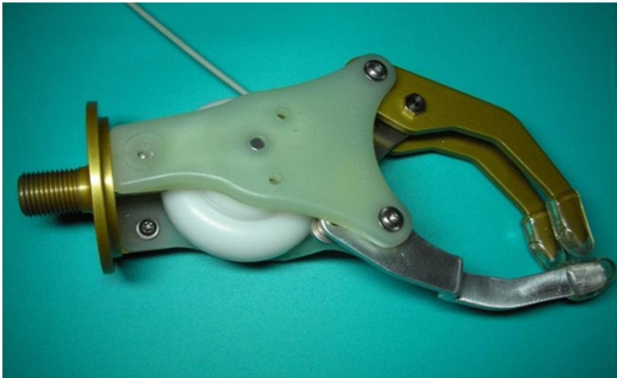
Fig. 13.4. Revised Otto Bock® Hand, Containing Extended Thumb.
