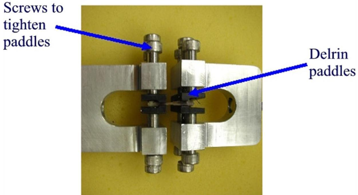
Fig. 13.1. Tensile Test Fixtures Holding a Murine Tibia.
