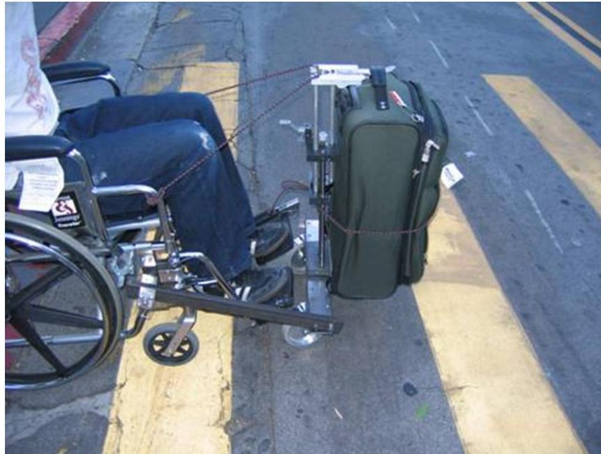
Fig. 10.6. Prototype of Luggage Assist Device.
