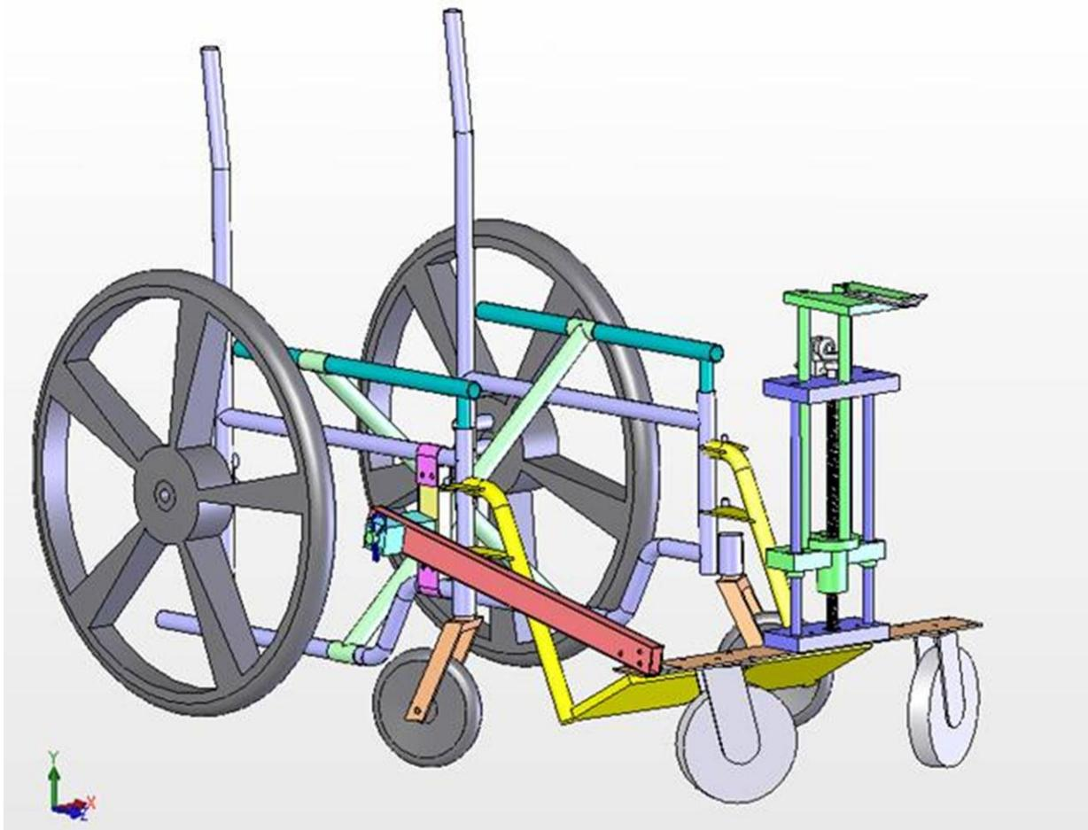
Fig. 10.5. CAD Model of Wheelchair Luggage Assist Device.
