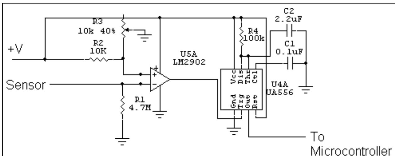
Fig. 20.3. Impact Detection Circuit.
