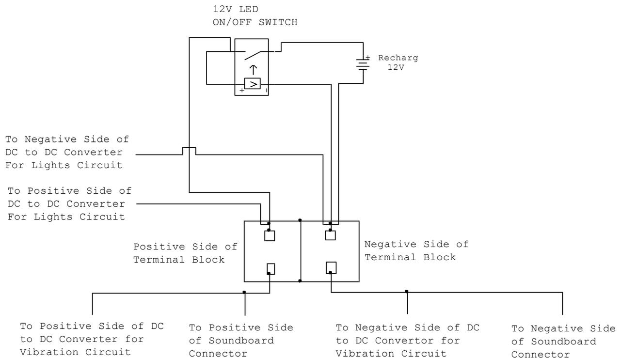
Fig. 20.11. Circuit Diagram of On/Off Switch and Terminal Board
