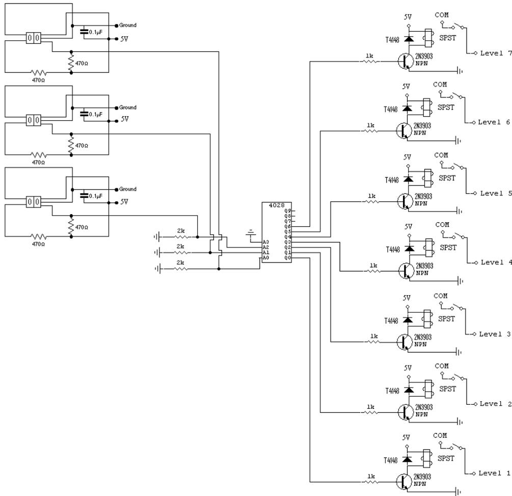
Fig. 20.6. Project Circuit Diagram.
