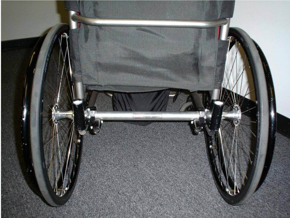
Fig. 13.3a. Rear View of Client's Wheelchair Shows the Open-ended Tubes Used to Attach the Trailer Ball Connector.
