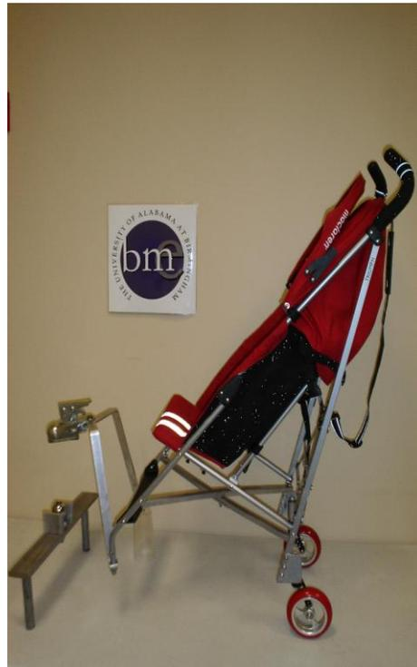
Fig. 13.3b. Adapted Stroller with Trailer Hitch and Trailer Ball Connector.
