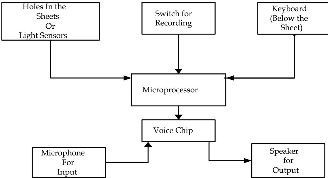
Figure 19.2. Block Diagram of the Communication Assist Device.
