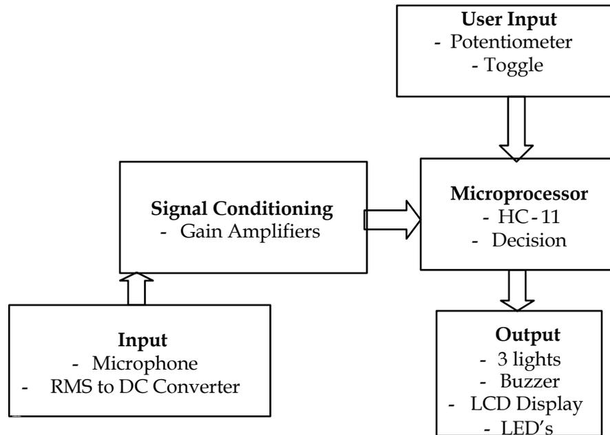
Figure 19.1. Block Diagram of Classroom Noise Level Indicator.
