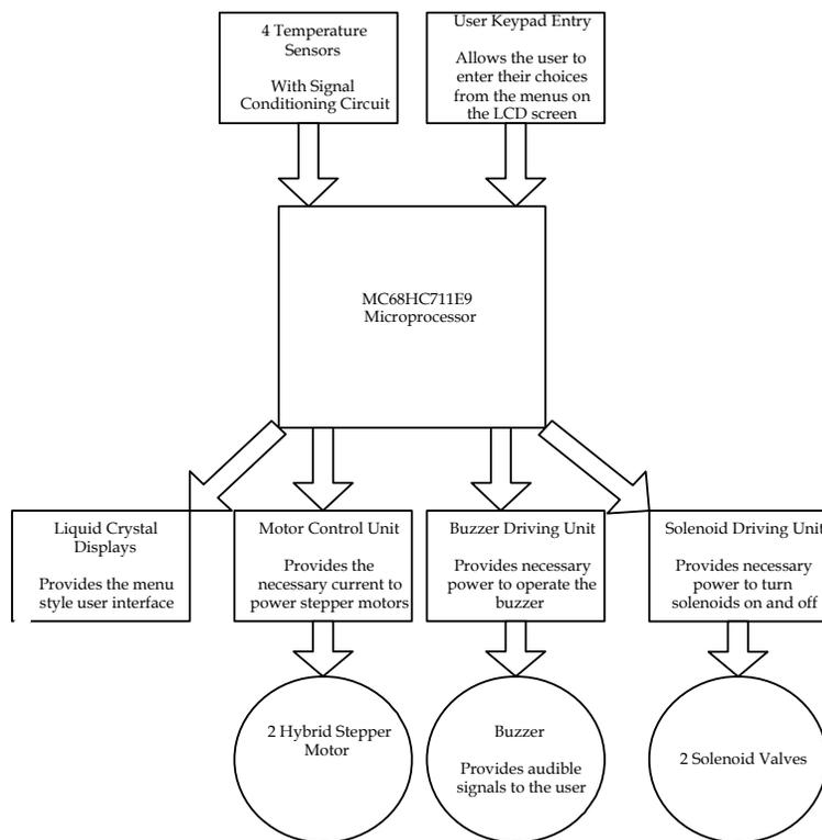
Figure 19.5. Block Diagram of the Digital Shower Temperature Controller.
