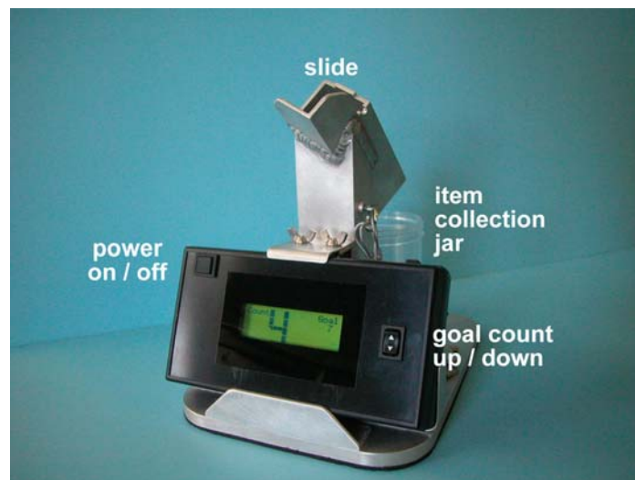
Figure 16.3 Assembled Small Item Counter with Templates Placed Over the Opening of the Slide.
