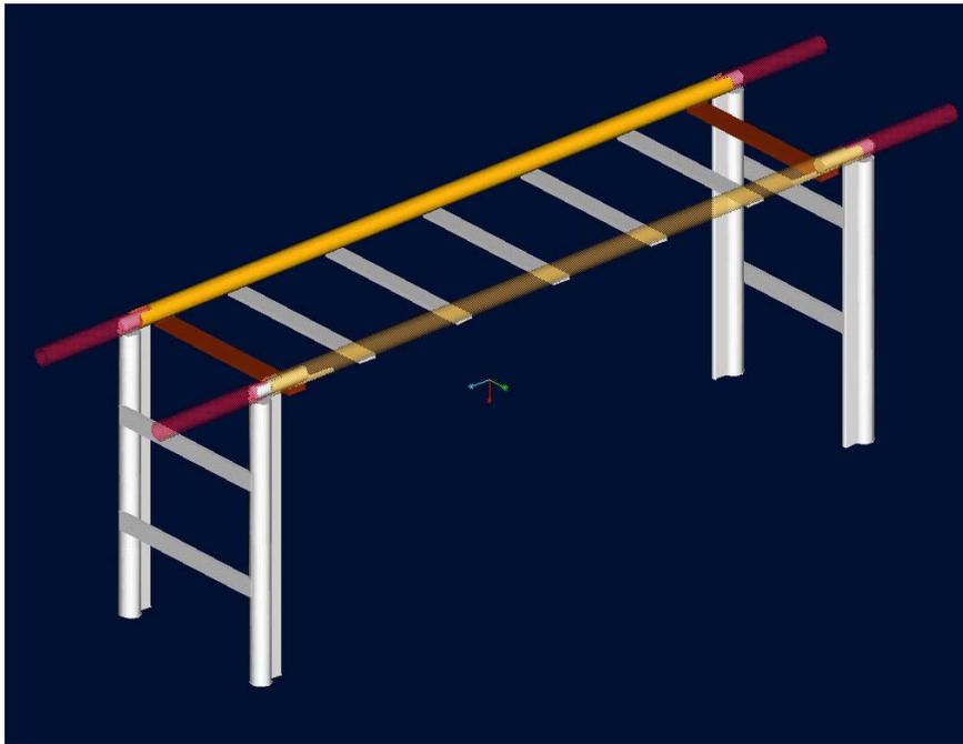
Figure 11.2. Drop-down Portion (yellow) of Motorized Drive.
