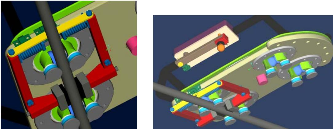
Figure 11.6. (Right) Bogey Riding on a Track Rail. (Left) Lock Pin for Rotating Plate.
