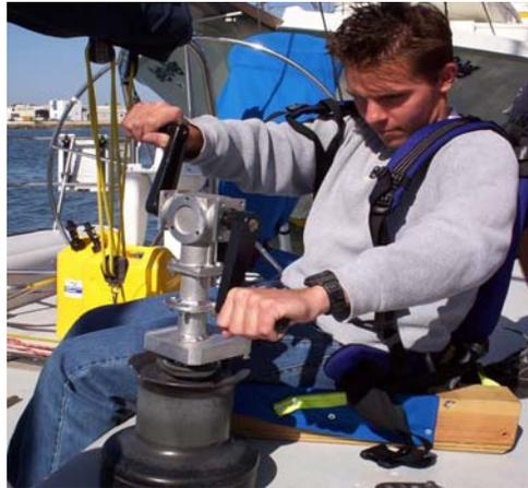
Figure 11.12. Winch-top grinder in use on a racing sailboat.
