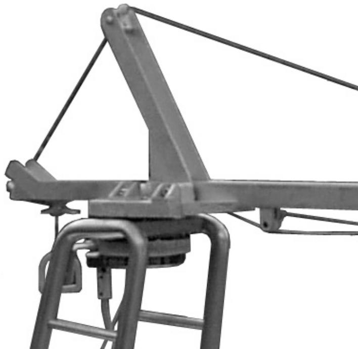
Figure 11.9. Turret and Furling Mechanism Close-up.
