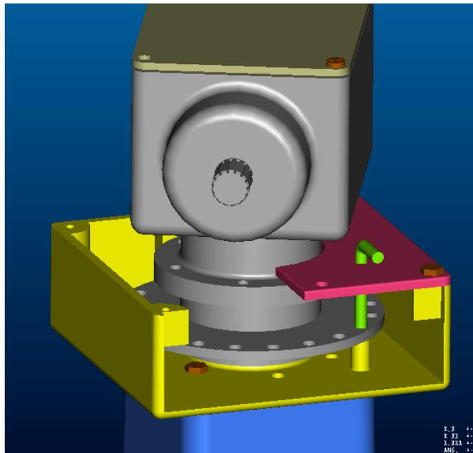
Figure 11.11. Gearbox and Rotating Mechanism Assembly Drawing.
