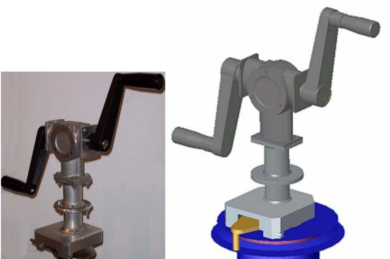
Figure 11.13. Winch-Top Grinder: Fabricated Prototype (left) and CAD Assembly Drawing (right).
