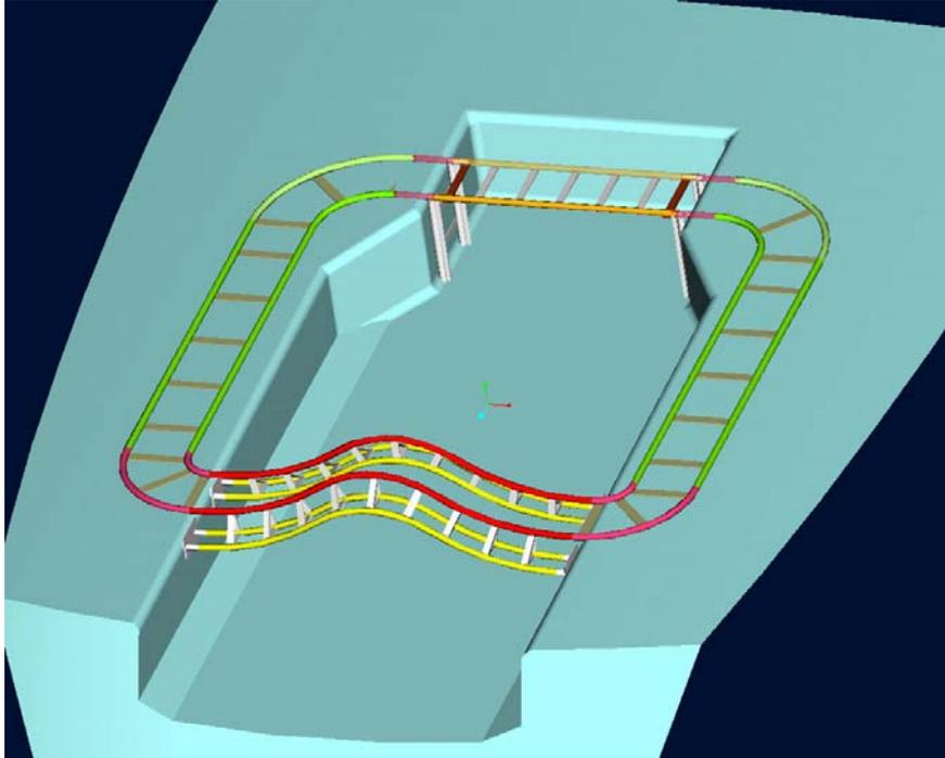
Figure 11.1. Twin Tubular Track Mounted on Cockpit.
