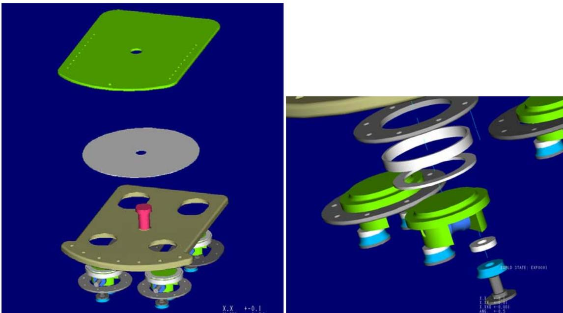
Figure 11.7. (Right) Trolley Underside with Brake. (Left) Trolley Underside with Brake and Brake Handle (cream & tan box).
