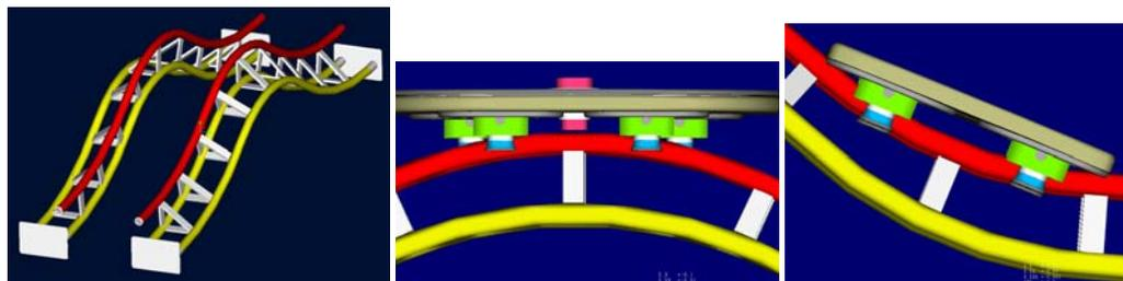
Figure 11.3. Arched Truss behind Helm (left), Check for Interference between Tube Rails and Bogeys of Trolley over Convex (middle) and Concave (right) Truss Sections.
