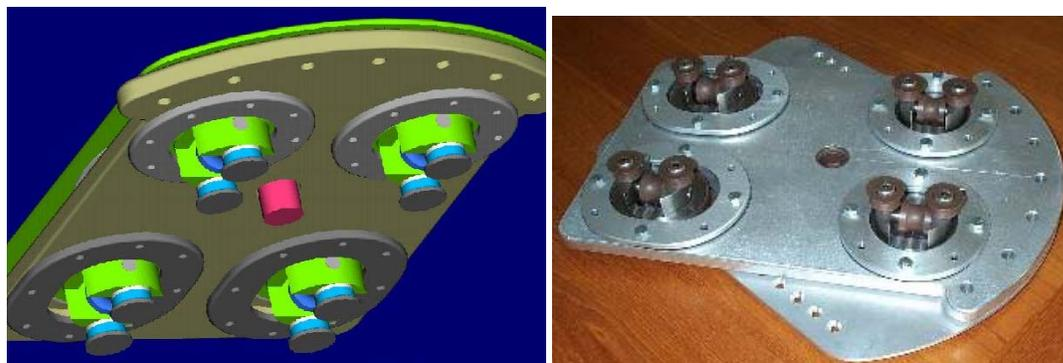
Figure 11.4. Trolley Underside with four Bogeys that Retain Trolley on Tracks (CAD Model, left; Prototype Hardware, right).
