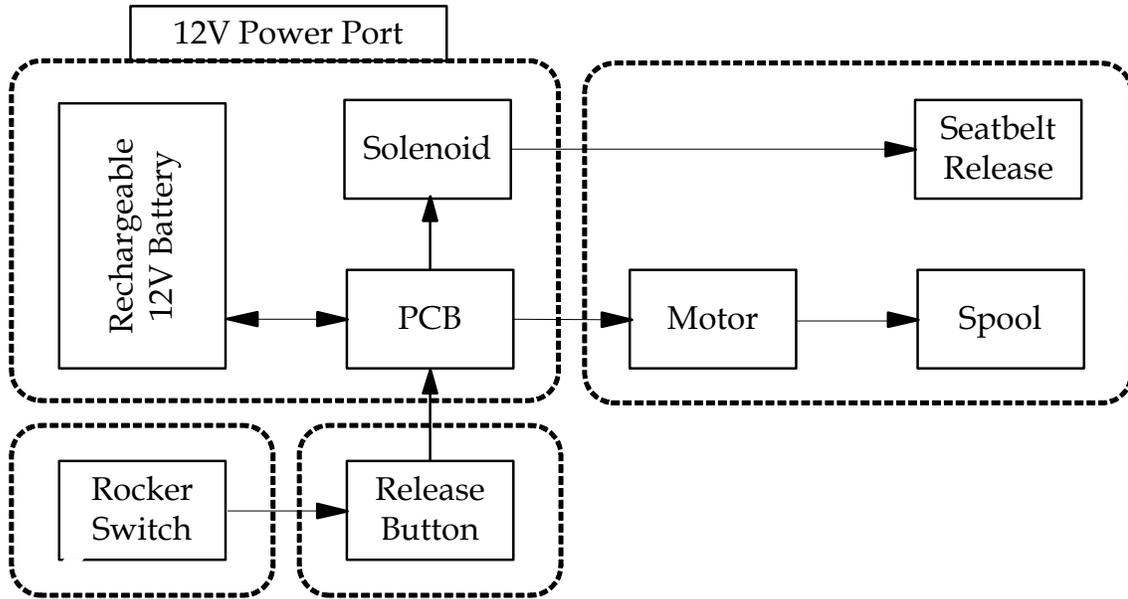
Figure 10.12. System Block Diagram.
