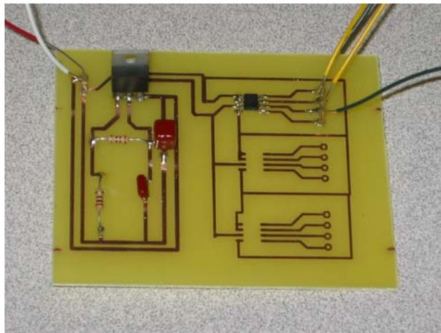
Figure 10.10. H-bridge Circuit.
