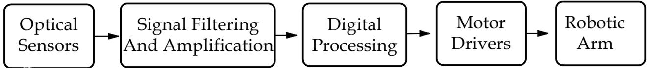
Figure 10.8. System Block Diagram.
