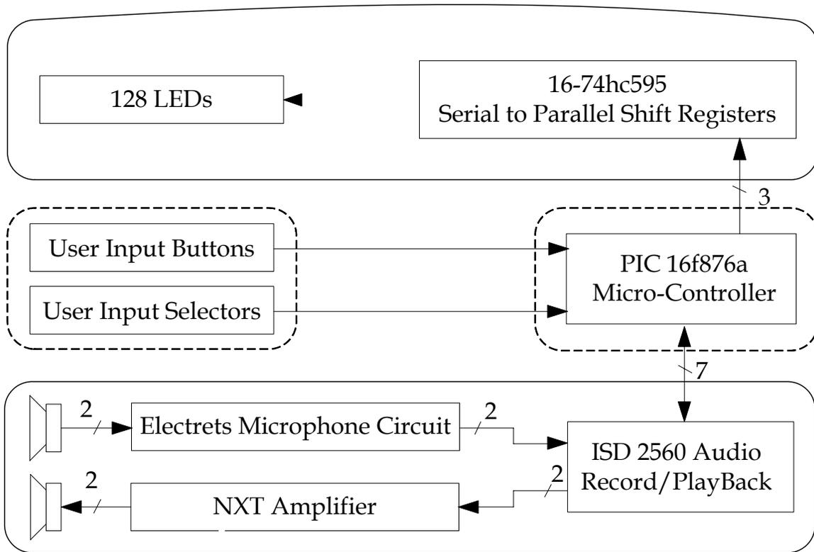
Figure 10.4. System Block Diagram.
