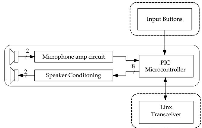
Figure 10.5. System Block Diagram.
