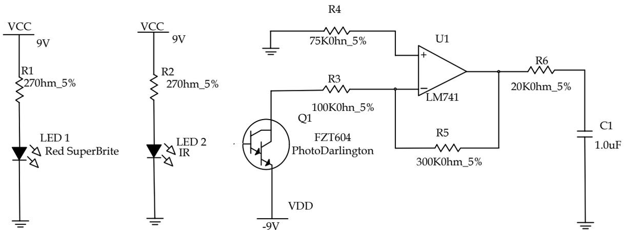
Figure 10.9. Sensing Unit Schematic..
