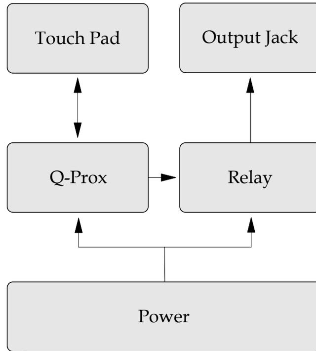
Figure 10.2. System Block Diagram.
