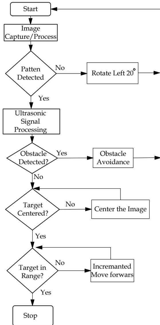
Figure 10.21. Wander Alert System Block Diagram.
