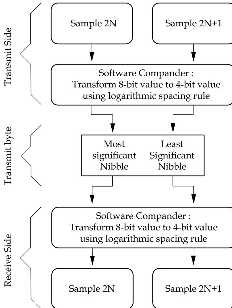
Figure 10.7. Data Flow Block Diagram.
