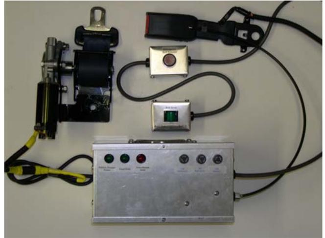
Figure 10.11. Assembled Hands-Free Seatbelt System.
