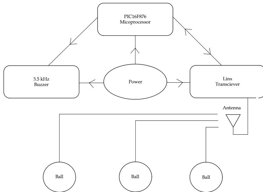
Figure 10.17. Block Diagram of Hub Component.
