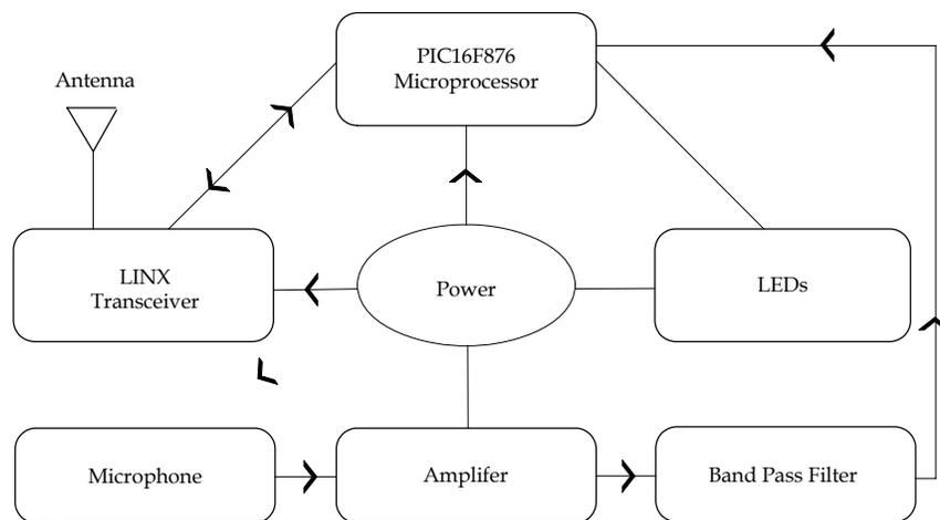
Figure 10.18. Block Diagram of Bocce Ball Component.
