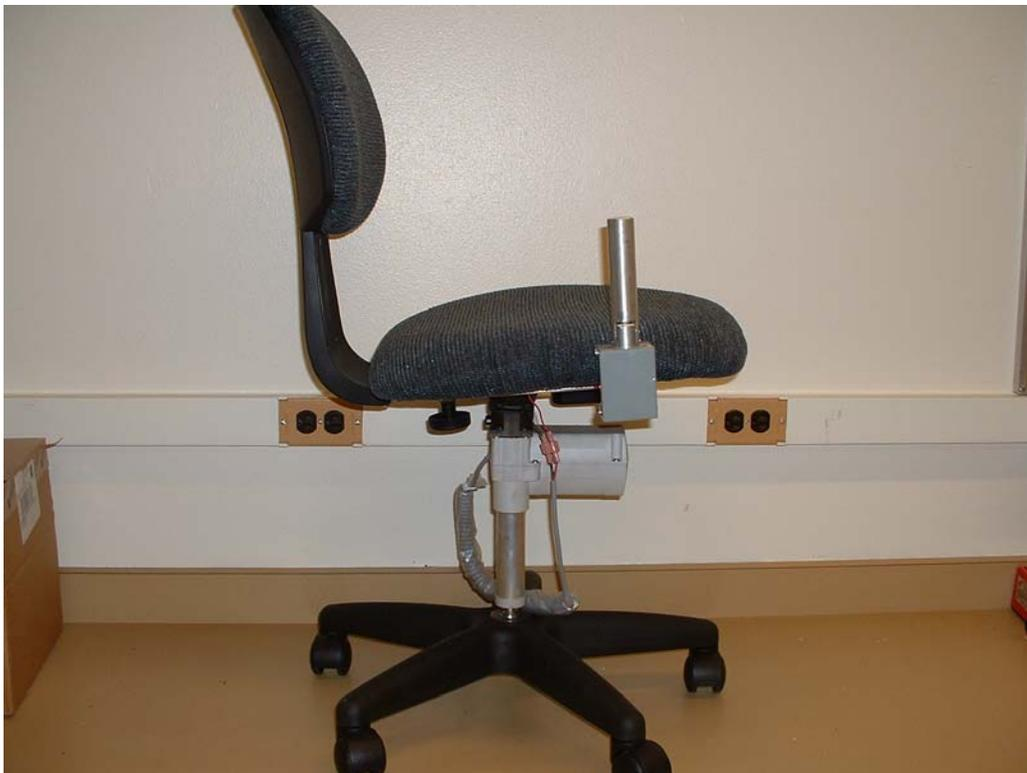
Figure 21.13. Raising and Lowering Control Using Enhanced Lever Arm (Joystick).
