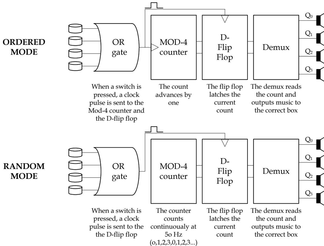
Figure 17.8. Block Diagram.
