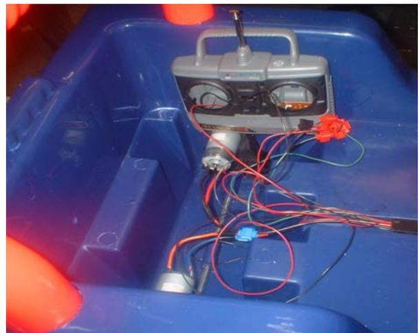
Figure 19.5. Connection for Speed and Receiver Control.
