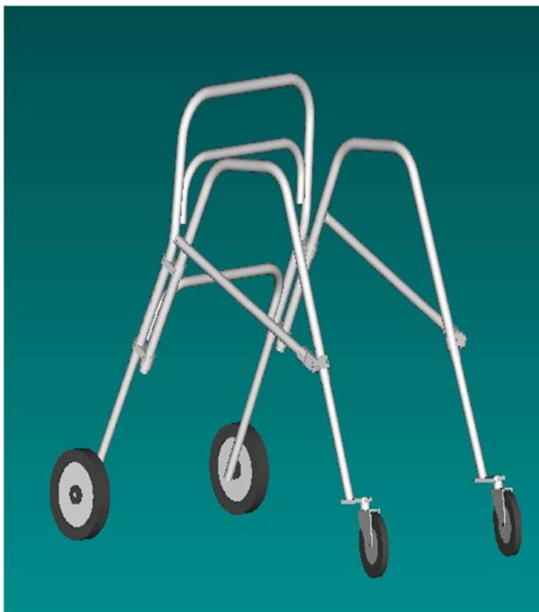
Figure 19.2. Re-designed Weight Assist Walker.
