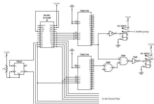
Figure 21.3. Output Electrical Circuit.
