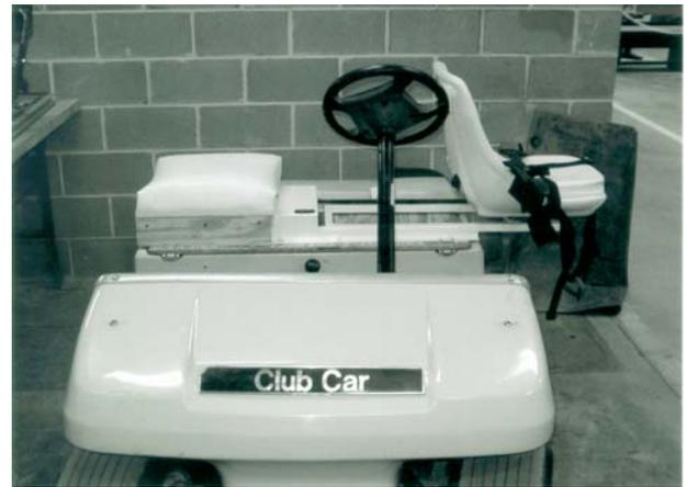
Figure 11.2: Seat Assembly in Playing Position.
