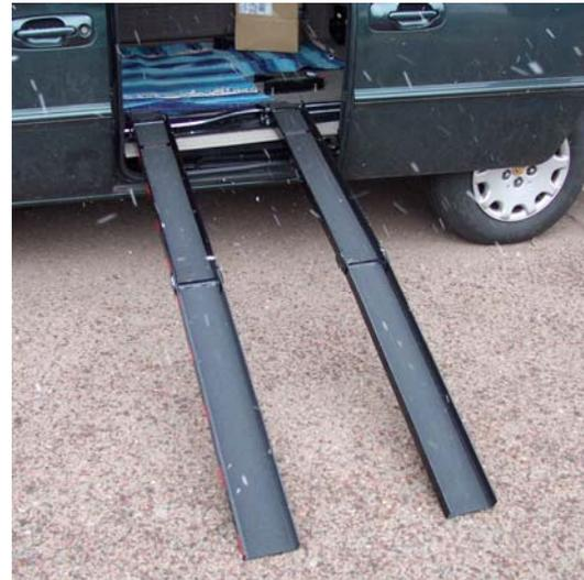
Figure 8.6. Fully Extended Wheelchair Ramp.
