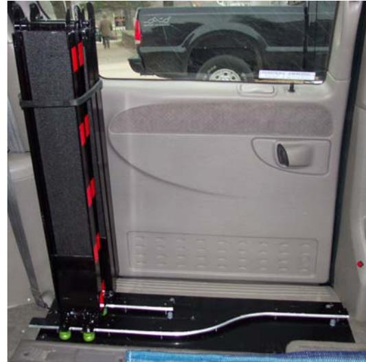
Figure 8.7. Wheelchair Ramp in Storage Position.
