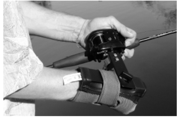
Figure 6.7. The Freshwater FRAD Attached to a Fishing Reel Handle.
