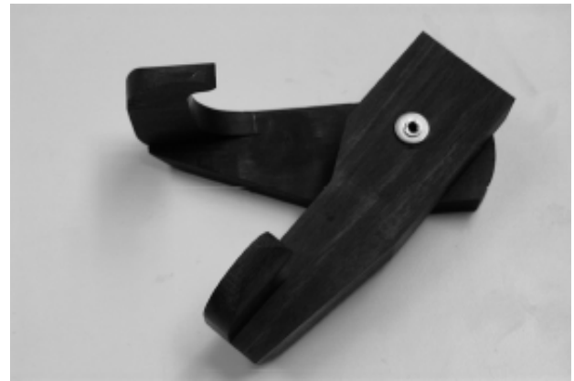
Figure 6.4. Split-Hook Prosthesis with Grasping Ability.
