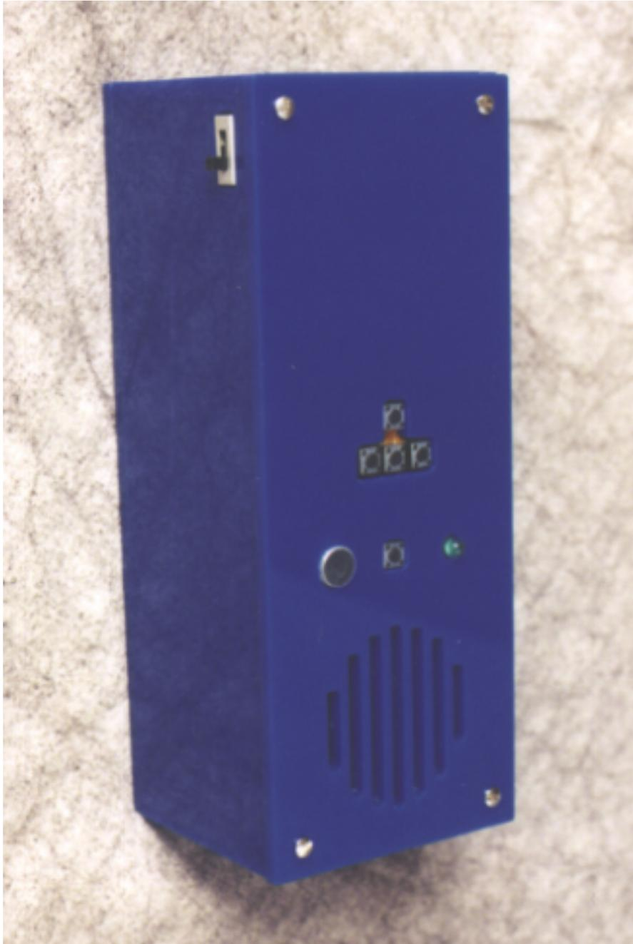
Figure 11.2. Digitally Secured RF Controlled Outlet.
