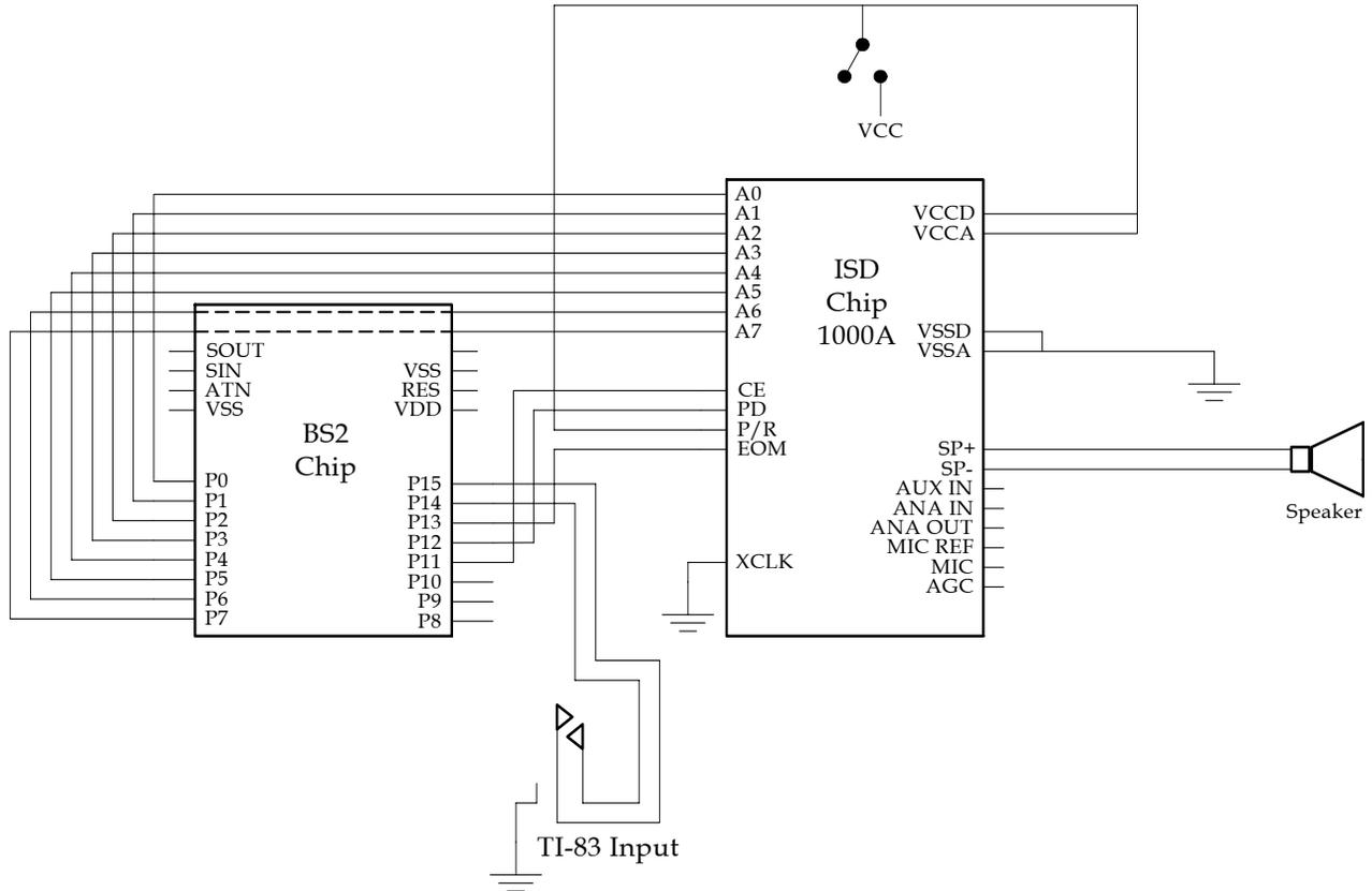
Figure 8.2. Voice Output Components.
