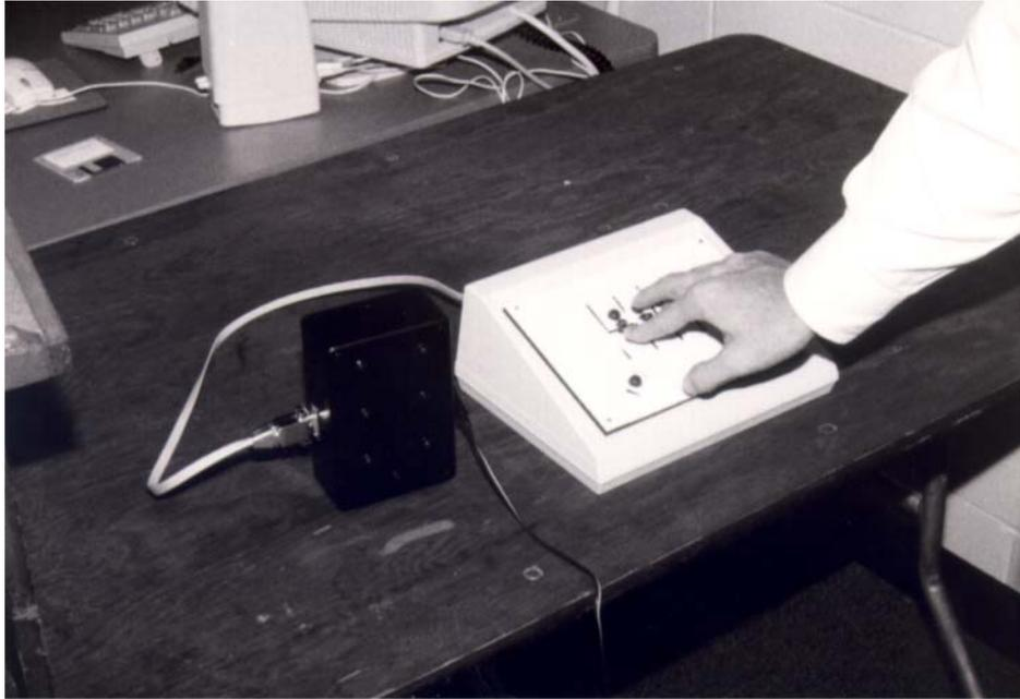
Figure 8.3. One-Handed Braille Keyboard.
