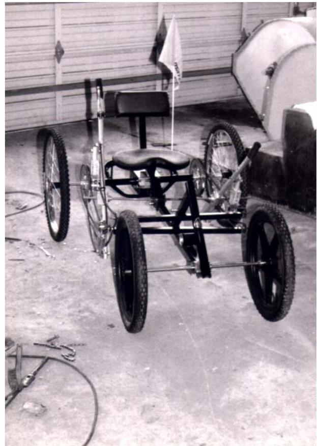
Figure 8.4. Chain-Drive Mechanism for an Off-Road Wheelchair.
