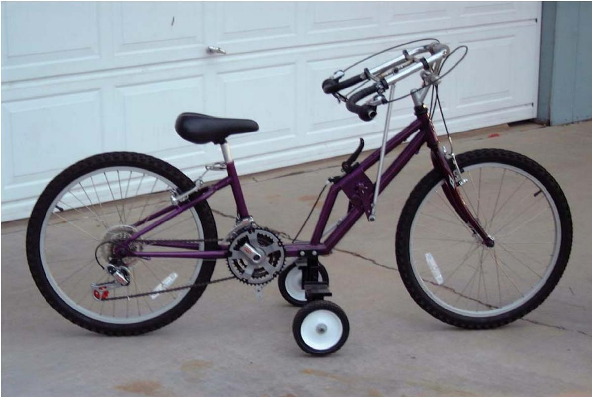
Figure 5.8. Photograph of the Hand Pump Bicycle.
