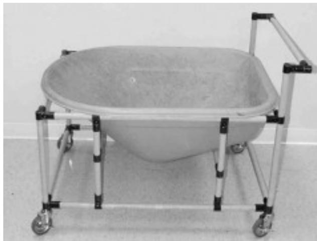
Figure 19.7. Material Handling Cart.
