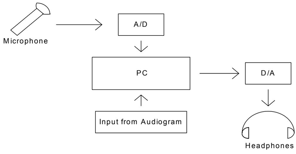
Figure 18.6. Hardware for Hearing Loss Simulator.
