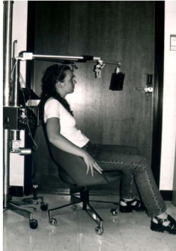
Figure 18.4. Tracking Device with Sensory Stimulation Card, Long (Far Left) and Short Vertical Shafts, and Enclosures (Center Left) Containing Power Supply, Circuitry, and Second DC motor.
