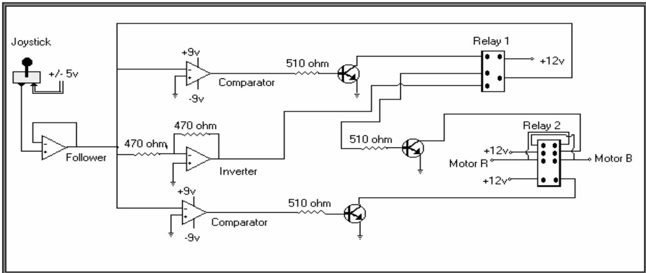
Figure 18.11. Wheel Propulsion Circuitry Located Under the Vehicle Seat.
