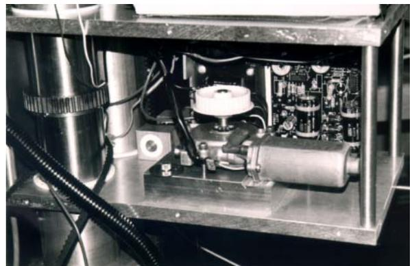
Figure 18.5. Enclosure with DC Motor in Foreground and Power Supply Behind.
