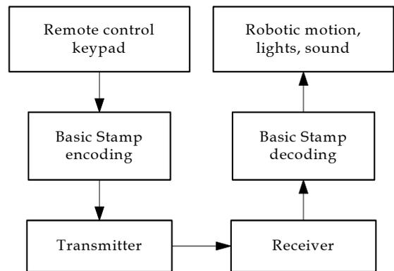
Figure 18.3. Block Diagram of Tracking Device.
