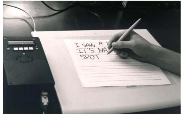
Figure 18.1. Interface Box (Left) with LCD display, Programmable Menu Switches, and LCD stimuli.
