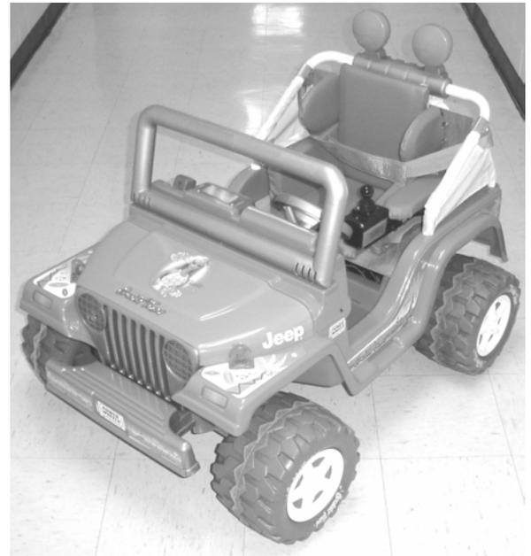
Figure 18.10. Modified Barbie Jeep with Supportive Seat and Joystick Control.
