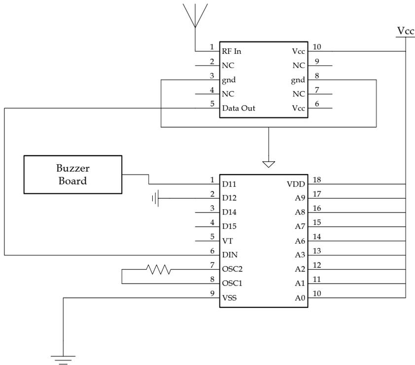
Figure 16.14. Receiver Circuit.
