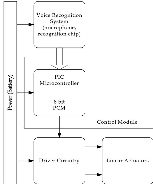
Figure 16.20. Block Diagram of E-GRIP.
