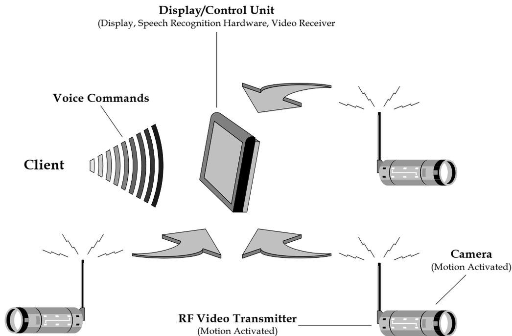
Figure 16.3. Components of the Speak-n-See Device.
