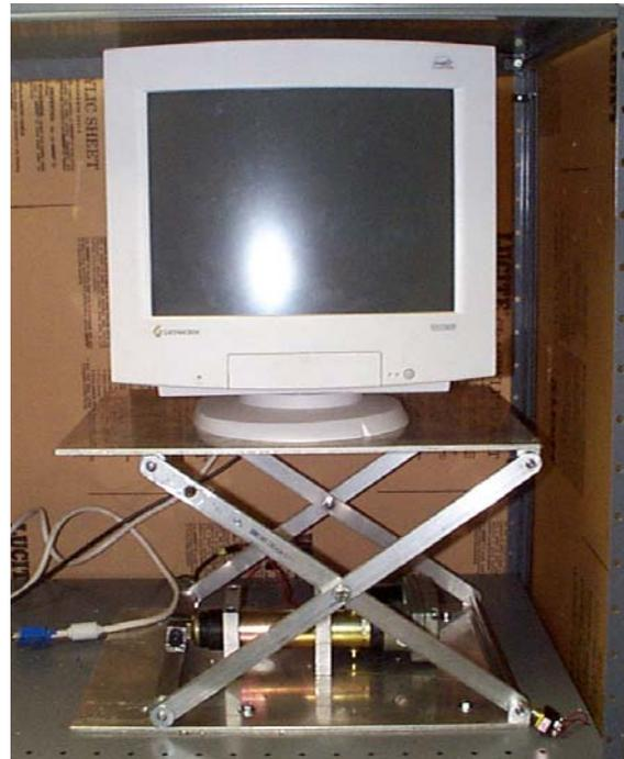
Figure 16.23. Monitor Lift inside the Roaming Diagnostic Station.
