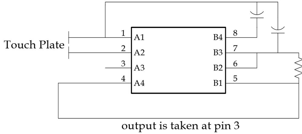
Figure 16.16. Touch Plate Circuit.
