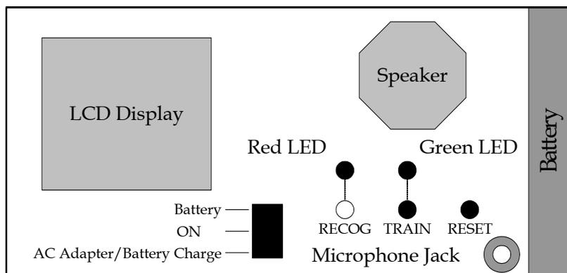
Figure 16.2. Display Unit Front Panel Layout.
