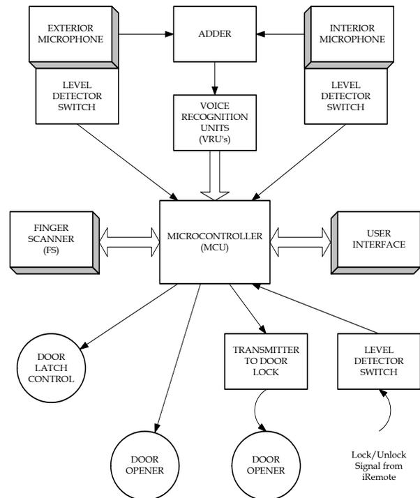
Figure 16.28. Functional Block Diagram.
