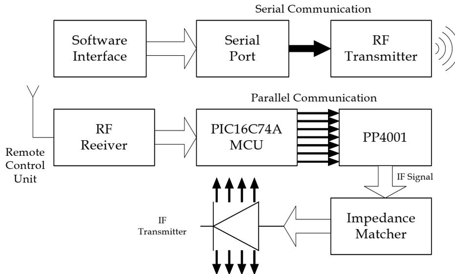
Figure 16.8. Block Diagram of the CERC.
