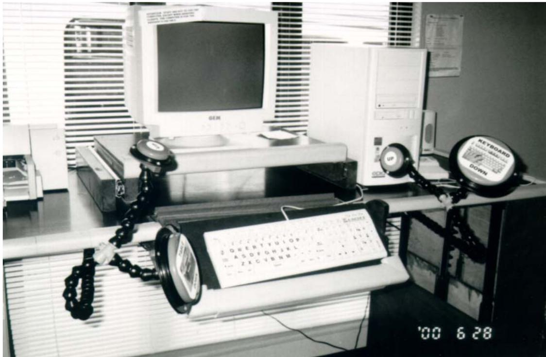
Figure 15.4. Close-Up View of Adjustable Computer Table, Showing Adjustable, Inclined Keyboard Tray, Sliding Monitor Stand and Jellybean Control Buttons.
