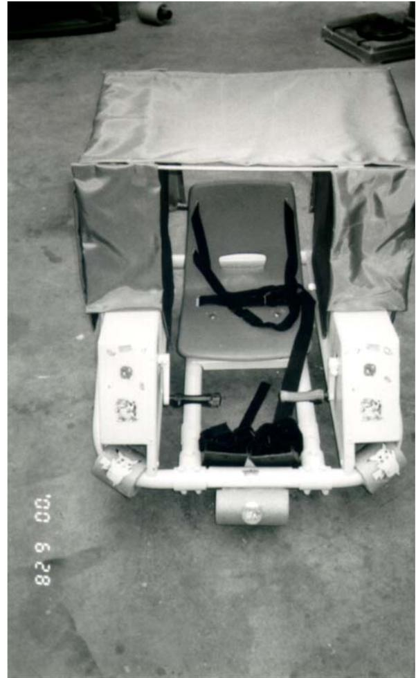
Figure 15.3. The Pokecart, Shown with Removable Canopy in Place.
