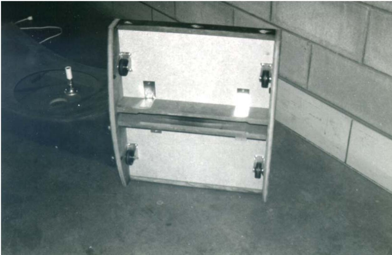
Figure 12.2 Top View of Platform Showing Slot and Curved Bottom.
