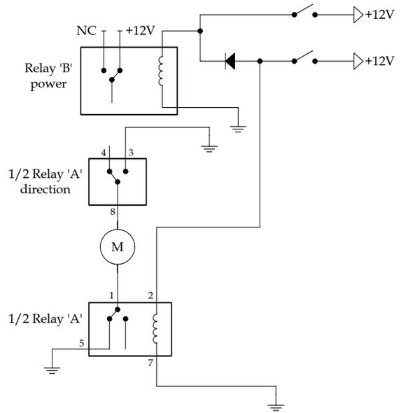
Figure 12.18. Circuit for Moving Gun in Horizontal Plane.
