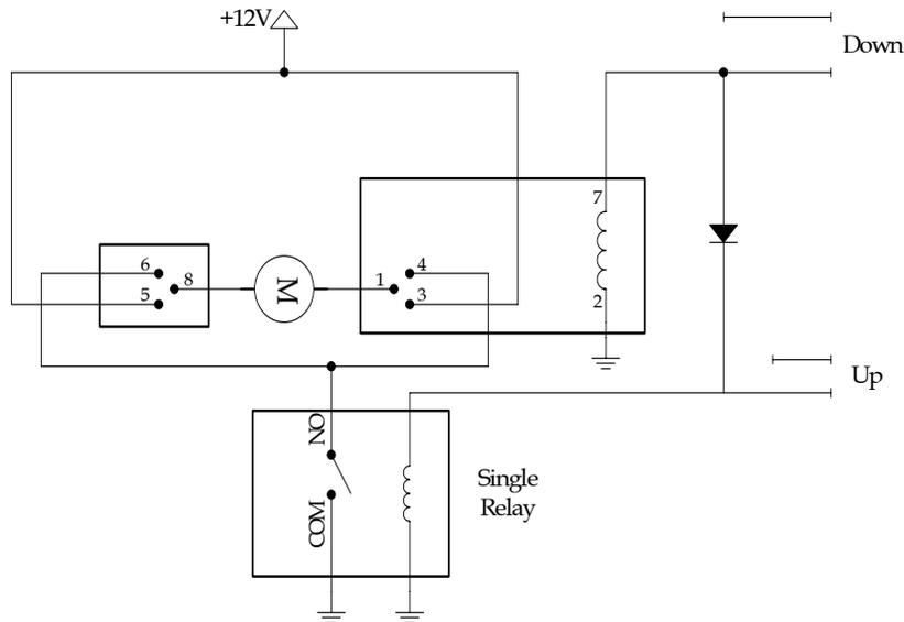
Figure 12.19. Circuit for Moving Gun in the Vertical Direction.
