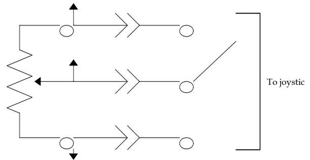
Figure 12.16. Airtronics Controller with Two Three-Terminal Potentiometers.
