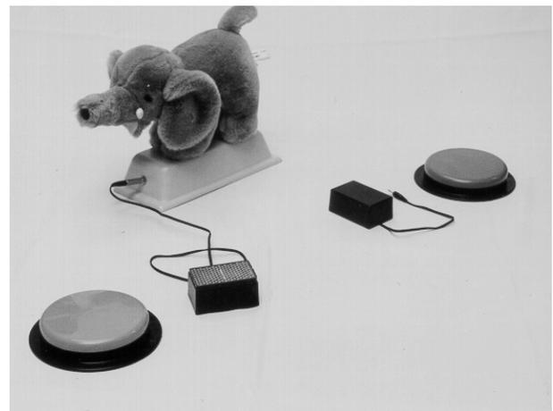
Figure 12.8. Water Shooting Toy with Two Cordless switches. Receiver Attached to Toy has a Solar Panel; the Other Uses Batteries.
