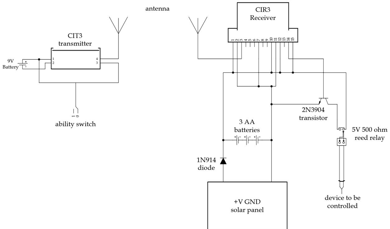
Figure 12.9. Circuit Diagrams of the Transmitter and Receiver.
