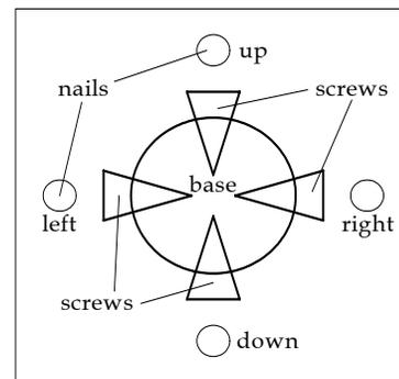
Figure 12.15. Schematic of Interface between controller potentiometer and the joystick.
