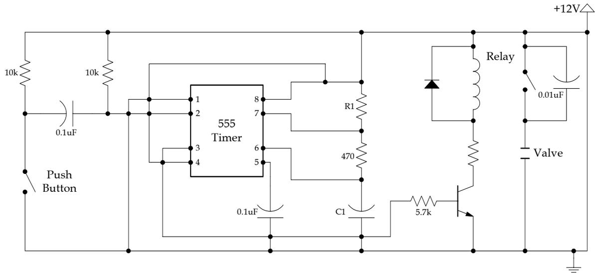
Figure 12.20. Timing Circuit for Gun Valve.
