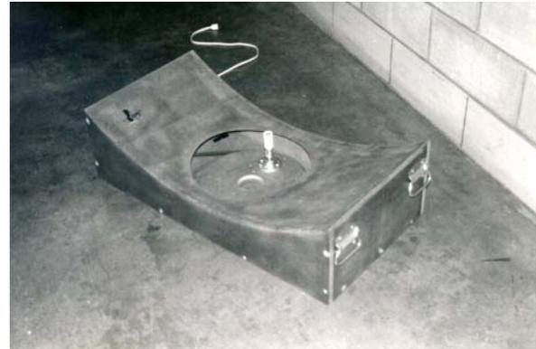
Figure 12.1 Base showing driver which fits in the groove at the bottom of the platform.
