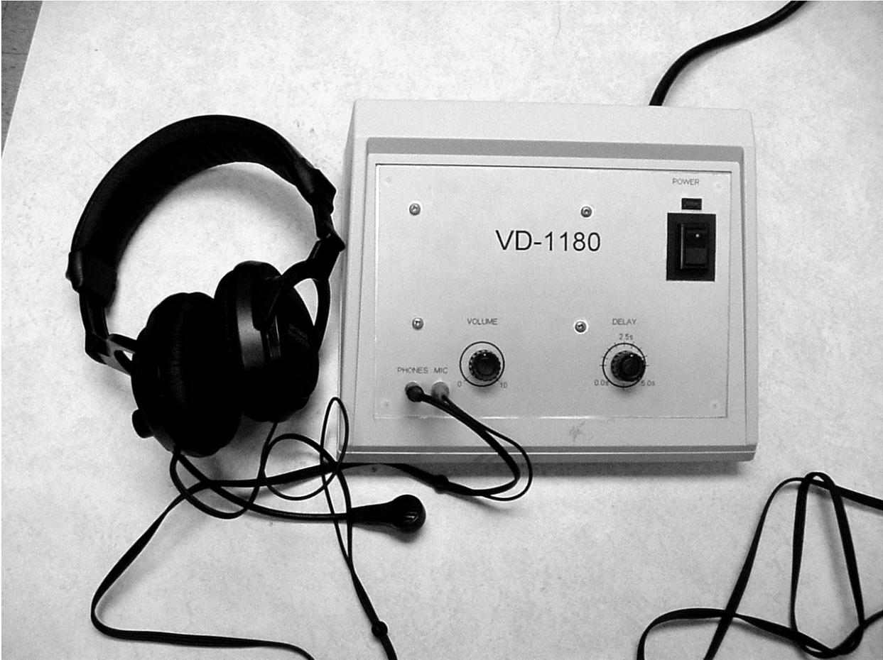
Figure 10.7: Final Voice Delay Device.
