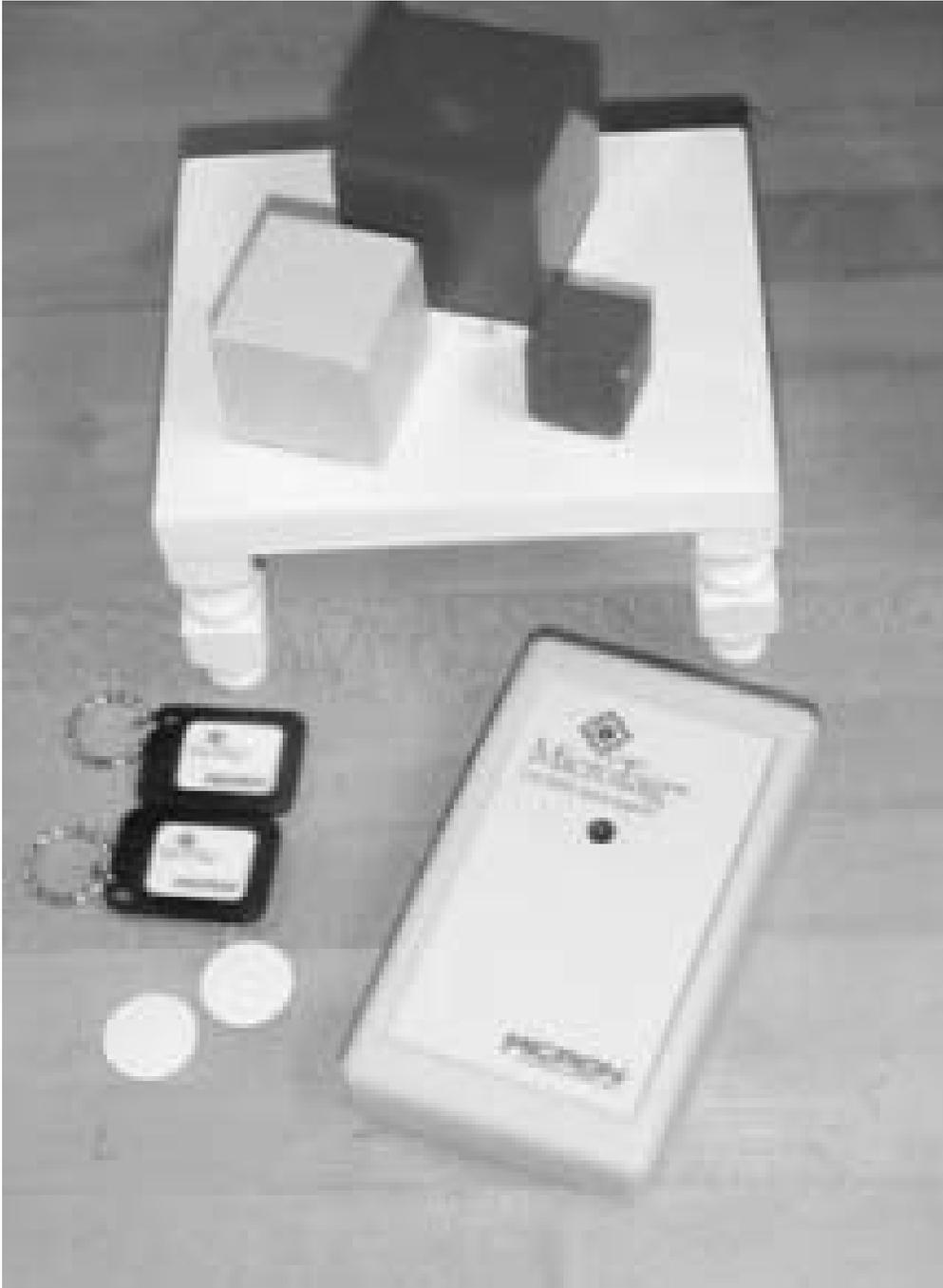
Figure 20.11. Micron RF MicroTag Reader, RF Tags, and Colored Blocks.
