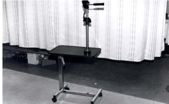
Figure 20.21. Augmentative Communication Device Mount.
