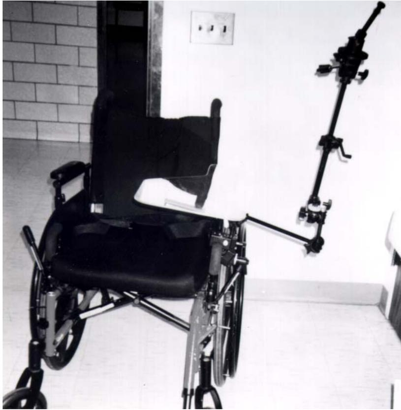
Figure 20.24. System Mounted on a Manual Wheelchair.
