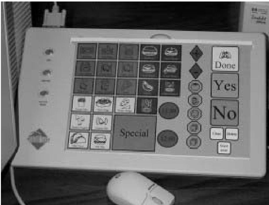
Figure 20.27. Intellikeys Touchpad with Custom Overlay.
