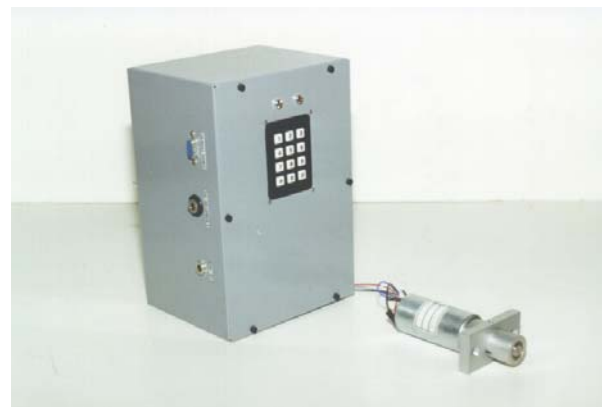
Figure 17.19. Electrolock. Shown is the keypad controller with the electronic deadbolt to the right.
