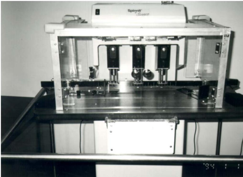
Figure 16.4. Close-Up of the Plexiglas Safety Cage, Showing the Hinged Doors and Magnetic Door Closers. The White Box Directly Beneath the Cage Houses the Secondary Electronic Circuit that Secures the Doors Closed During Operation.
