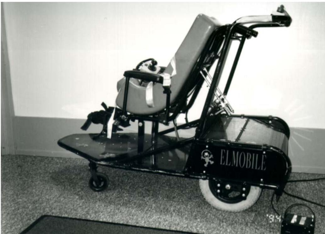
Figure 16.6. Side View of Elmobile, Highlighting Graphically Enhanced Fenders and Trunk, Housing Battery, Drive Assembly, Seat Tilt Mechanism, and Safety Switch.
