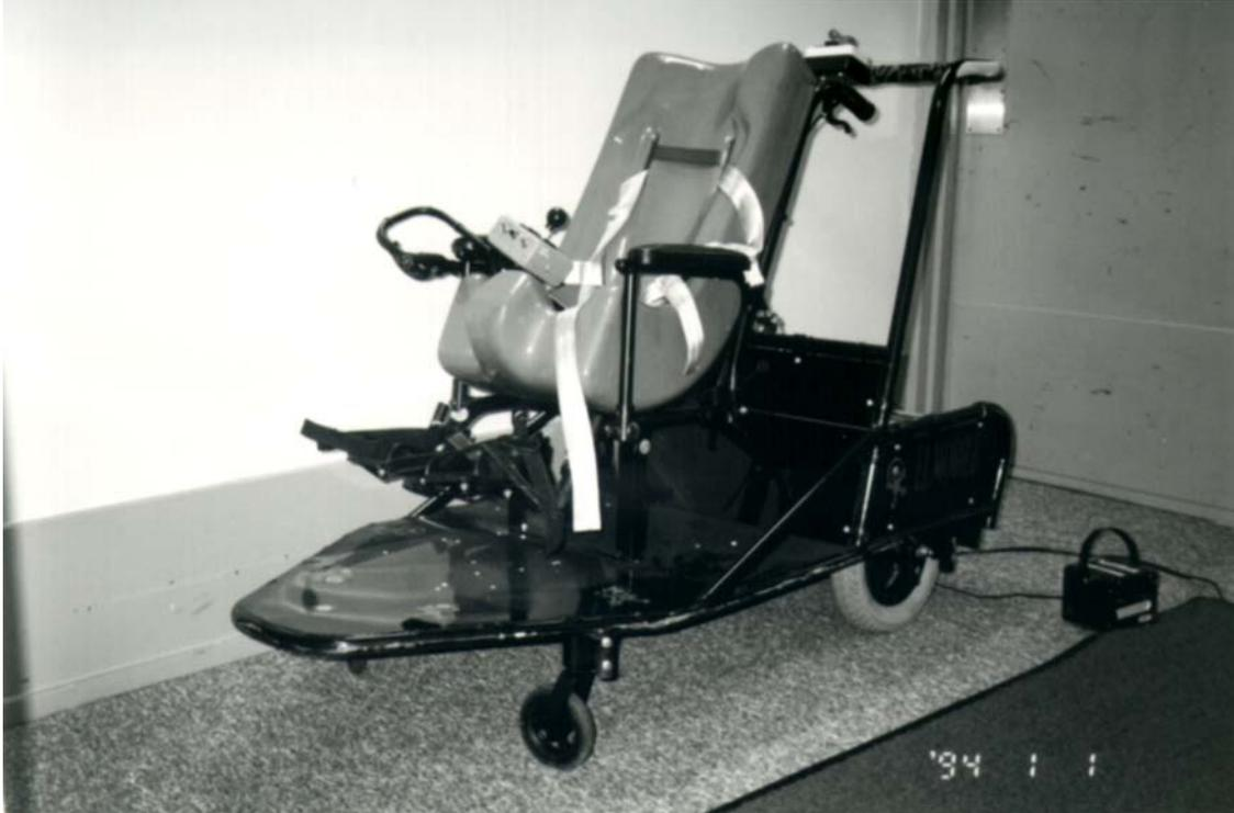
Figure 16.5. Front View of Elmobile, Showing Continuous Frame, Joystick Control, Safety Belts, and Footrests.
