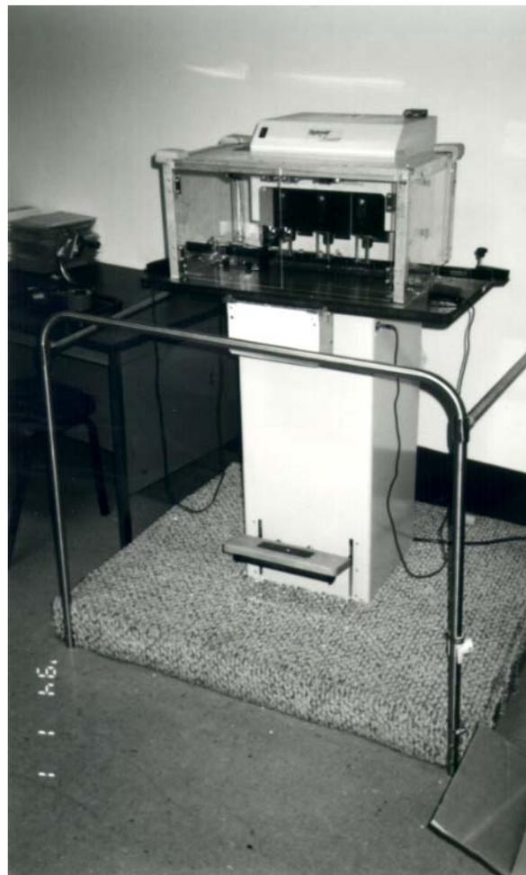
Figure 16.3. Modified Paper Drilling Machine with Plexiglas Safety Cage, Pallet Base and Guard Rails.
